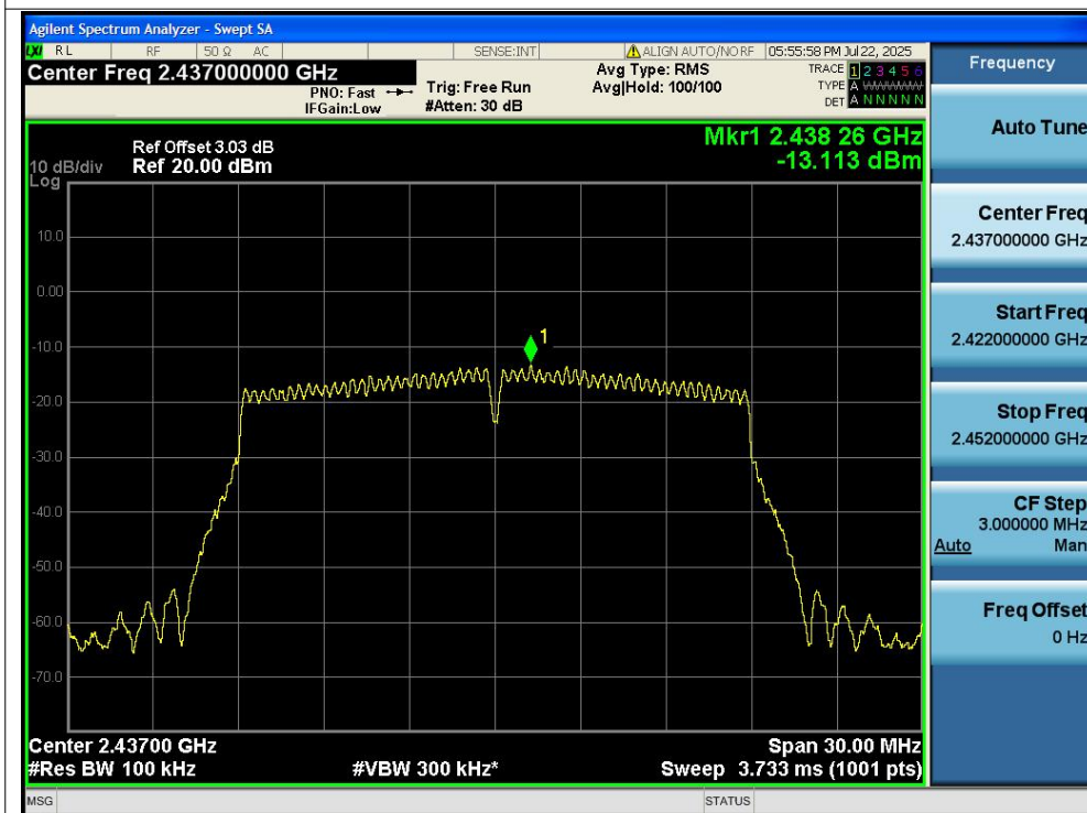
PSD NVNT n20 2437MHz Ant1
