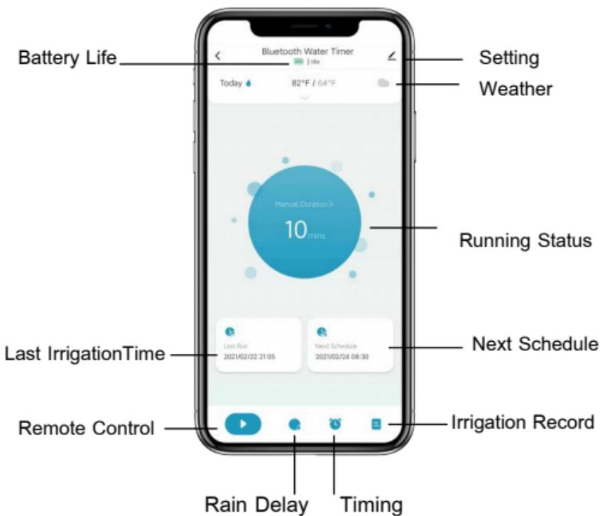
Press the "Timing" button and then the "+", you can set "Normal Schedule" or "Cycle/soak" watering program.
