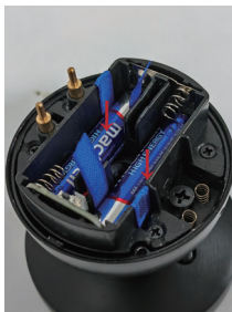
10. Install the next two batteries
