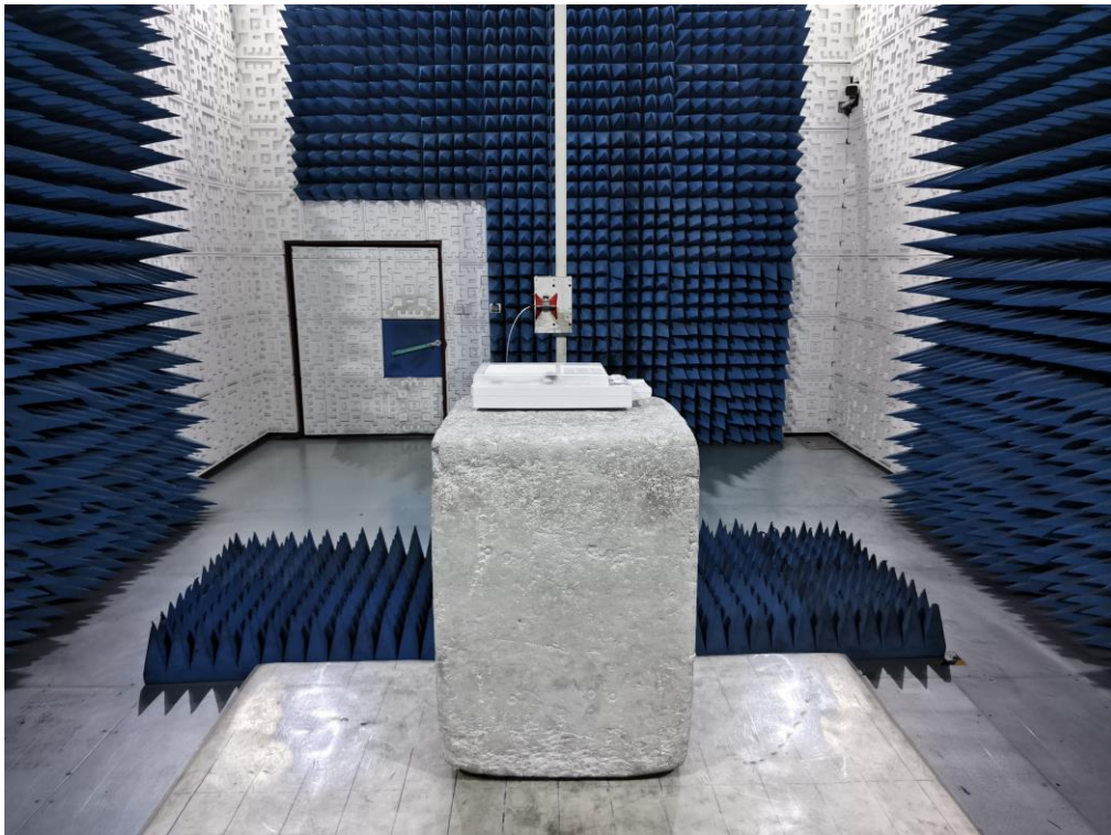
RADIATED EMISSION TEST SETUP ABOVE 1GHz
