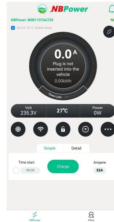
④You can view the current charging related values in the main control interface, start charging, stop charging and other functions, you can also make appointments for charging, current size adjustment settings
