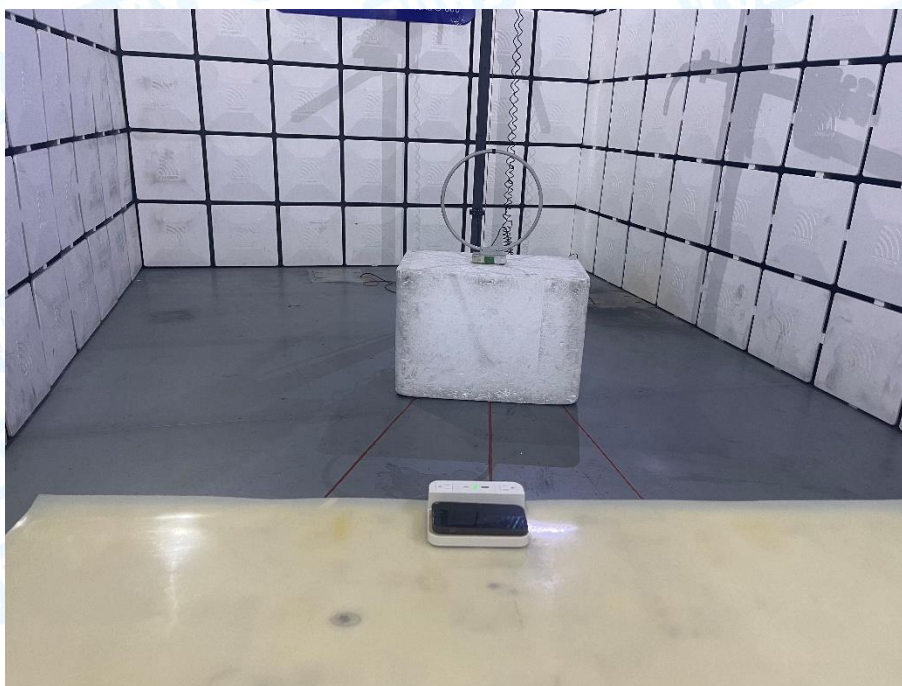
Photo of Setup for Radiated Emission (Below 30MHz)
