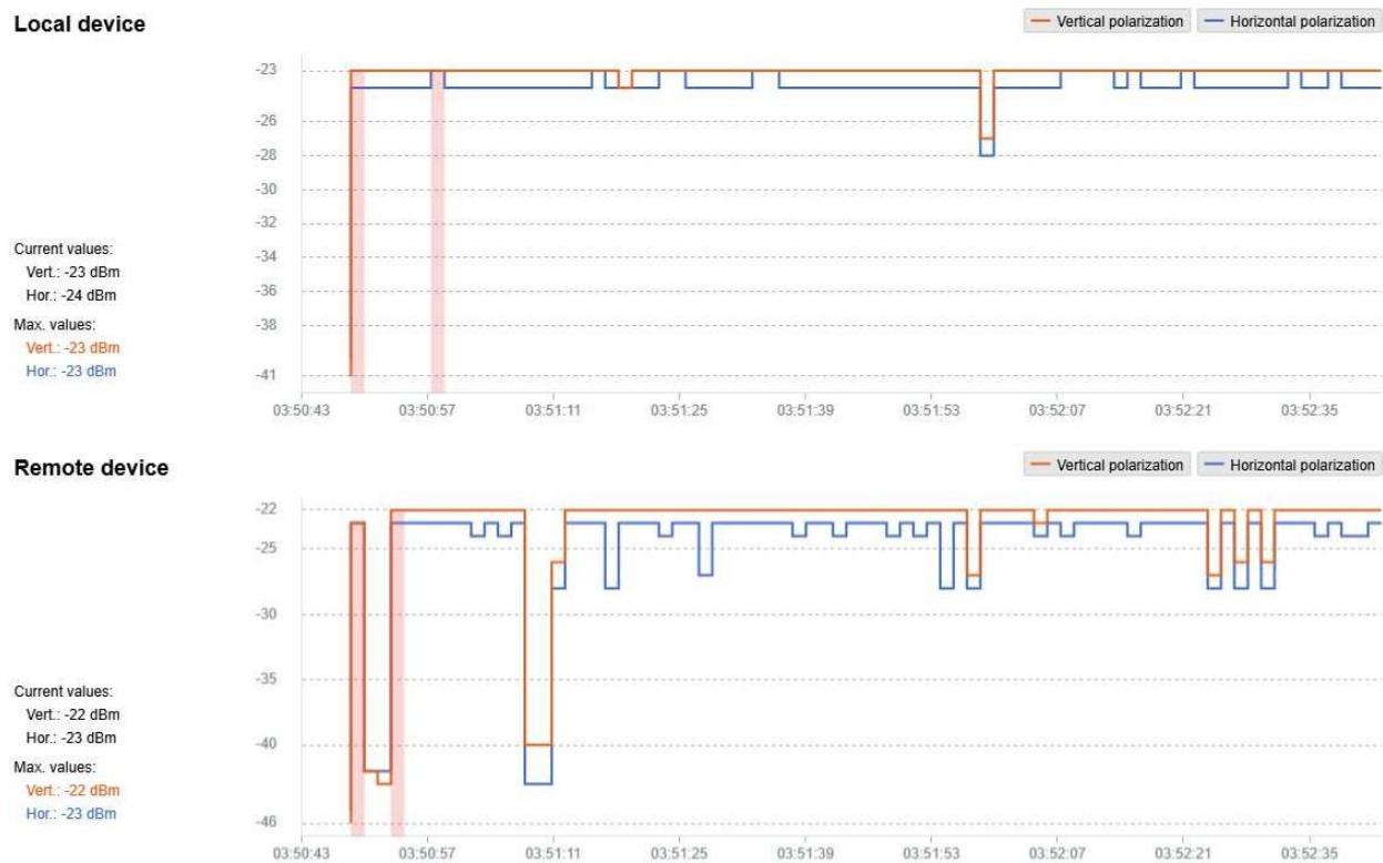
On the left edge of the graph there is a RSSI scale, below is a time scale (exact, if a connection to the SNTP server is performed or the time from the device being turned on). Red squares indicates break of the connection. Optimal RSSI values for operation at the highest modulations are -60...-40 dBm.
