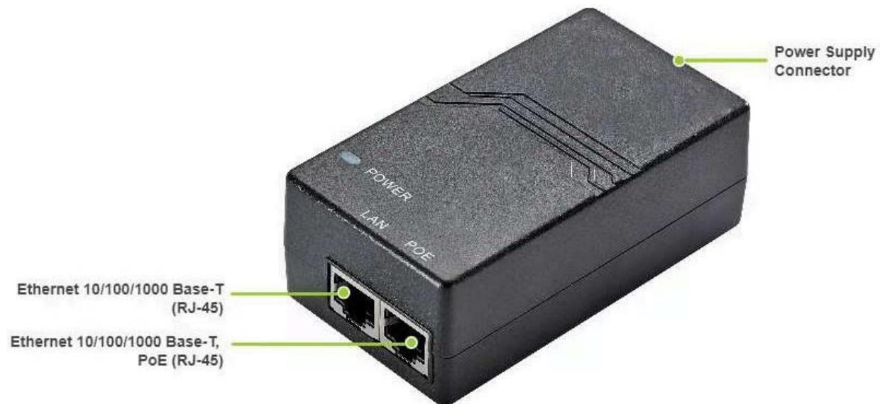
IDU-CPE-G(24W) is an indoor Gigabit PoE injector which supports 100-240 V input range from the AC mains. IDU-CPE-G(24W) feeds 48 VDC power to the device by injecting it to the CAT5 Ethernet cable.
