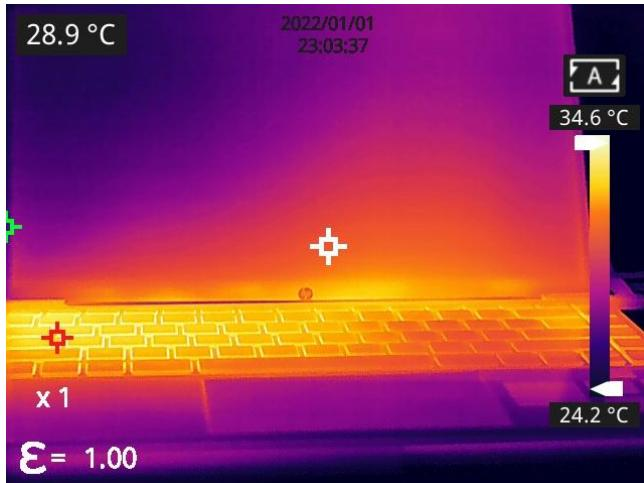
The lower limit of the temperature scale is manually adjusted as 27.7°C:
