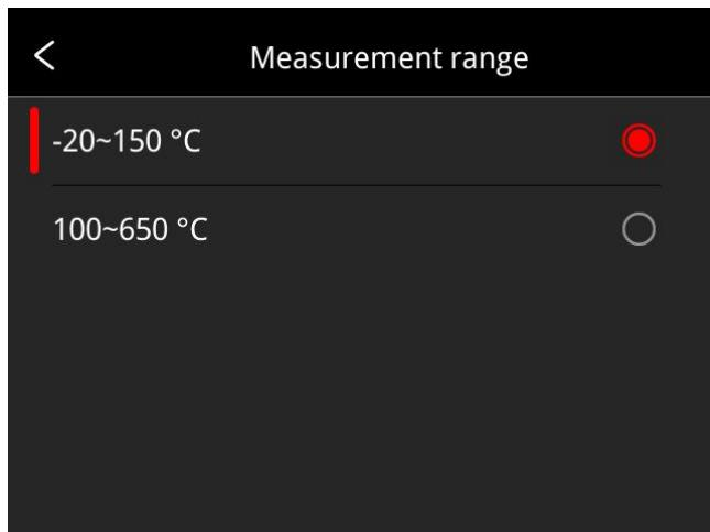
Select the options up-down by navigation button, press OK to confirm; You can also select the options via the touch screen.
