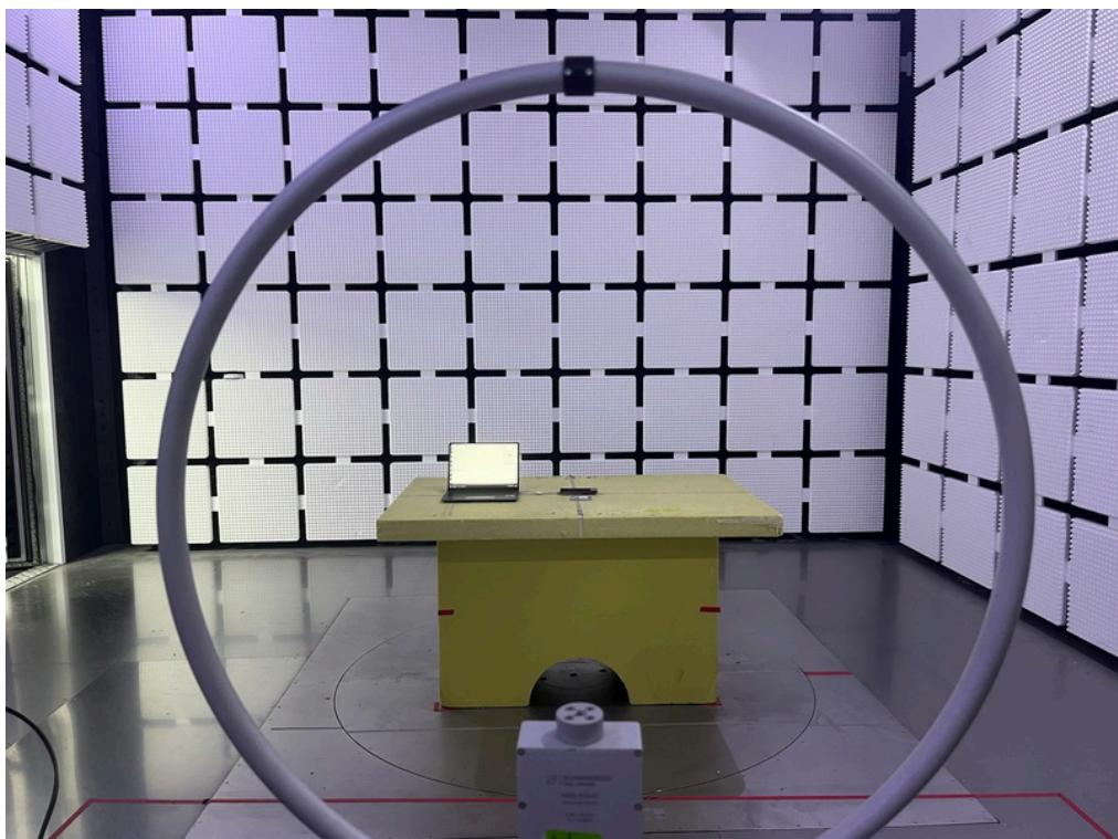
**Radiated Emissions Test Photos****30 MHz to 1000 MHz**
