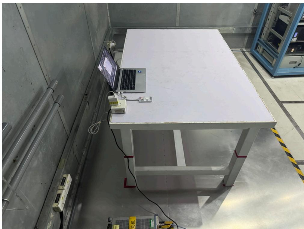
**Radiated Emissions Test Photos****9 kHz to 30 MHz**
