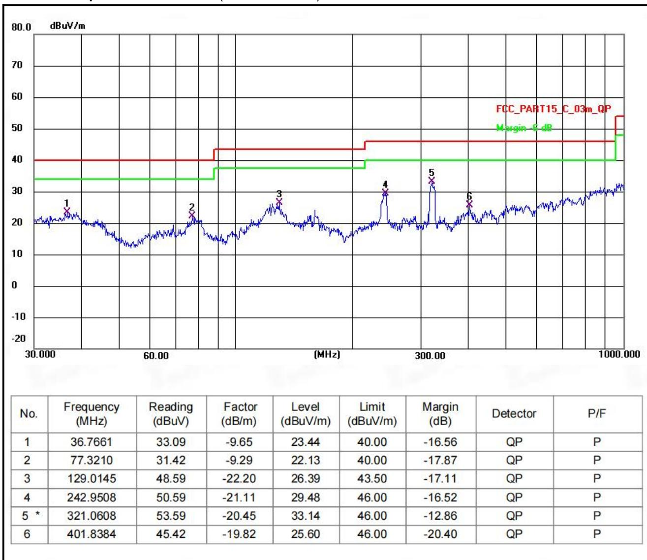
Note: Margin = Level - Limit = Reading + factor - Limit
