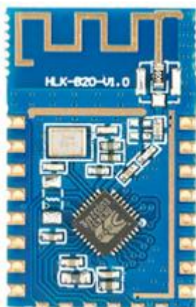
Figure 1: Position and schematic diagram of the onboard antenna on the HLK-B20 board
