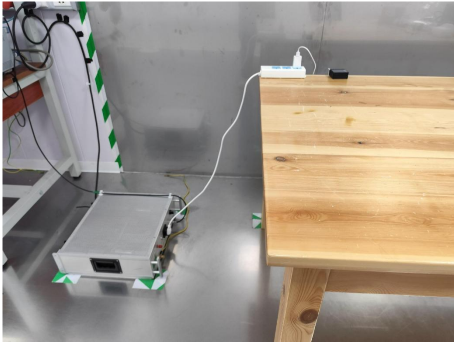
Conducted Emission at AC power line
