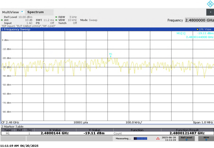
Figure 29: Power Spectral Density, BLE 2M-PHY, Mode H (2480MHz)
