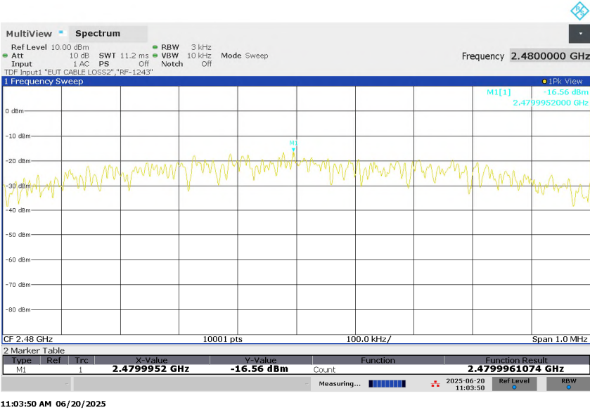
Figure 26: Power Spectral Density, BLE 1M-PHY, Mode H (2480MHz)
