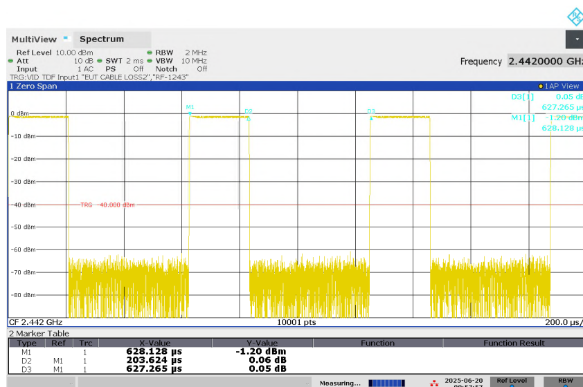
Figure 31: Duty Cycle, BLE 2M-PHY, Mode M (2442MHz)
