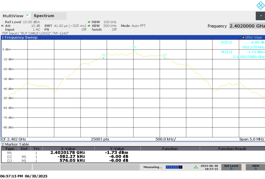
Figure 5: 6dB Bandwidth, BLE 2M-PHY, Mode L (2402MHz)
