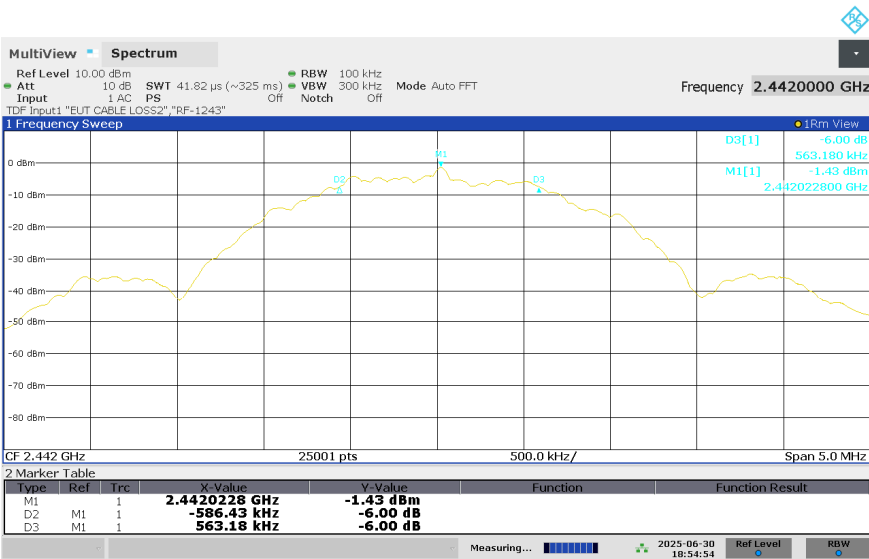
Figure 6: 6dB Bandwidth, BLE 2M-PHY, Mode M (2442MHz)
