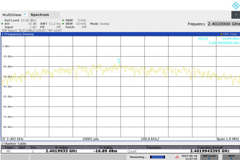
Figure 24: Power Spectral Density, BLE 1M-PHY, Mode L (2402MHz)
