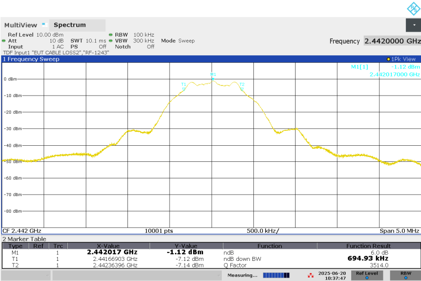
Figure 3: 6dB Bandwidth, BLE 1M-PHY, Mode M (2442MHz)
