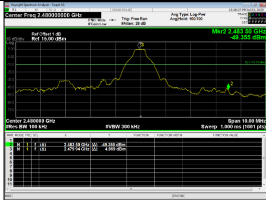
Out Of Band Emission GFSK_DH5_Channel 78
