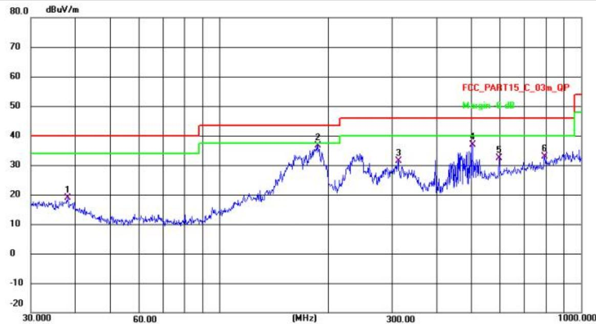
Note: Margin = Level - Limit = Reading + factor - Limit
