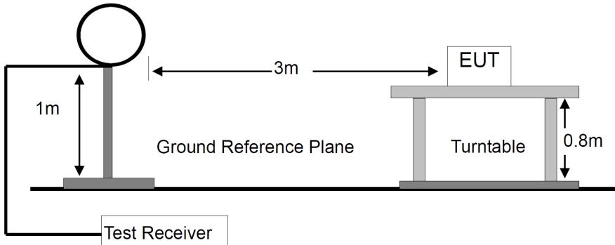
For Radiated Emission 30-1000MHz
