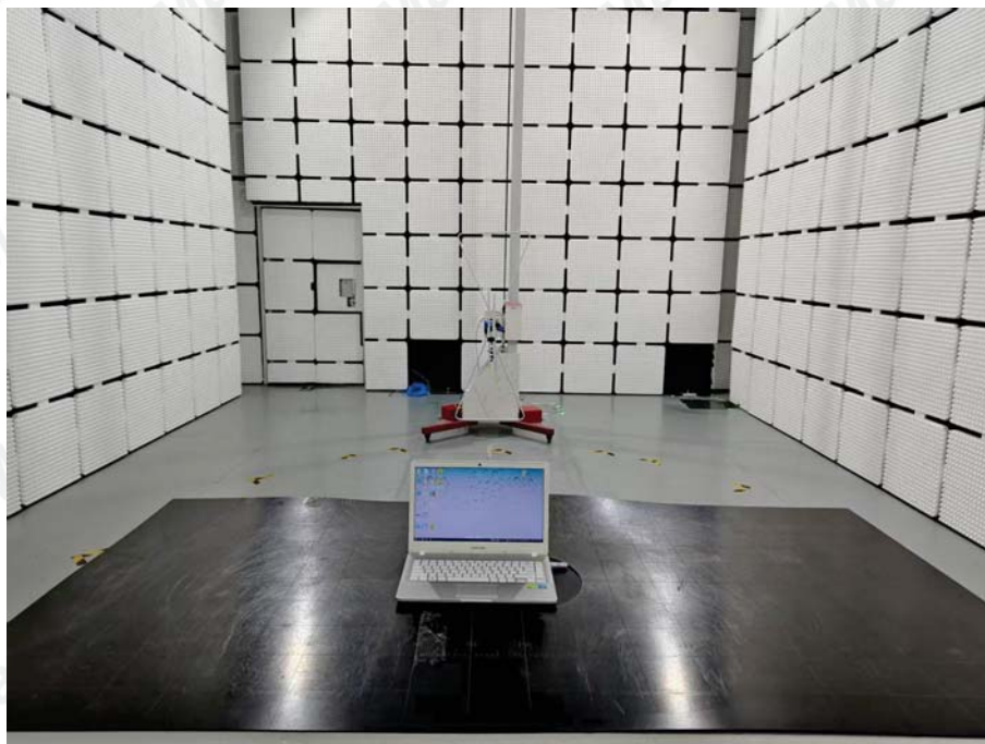
Photo 2 Radiated Emission Test (Above 1G)
