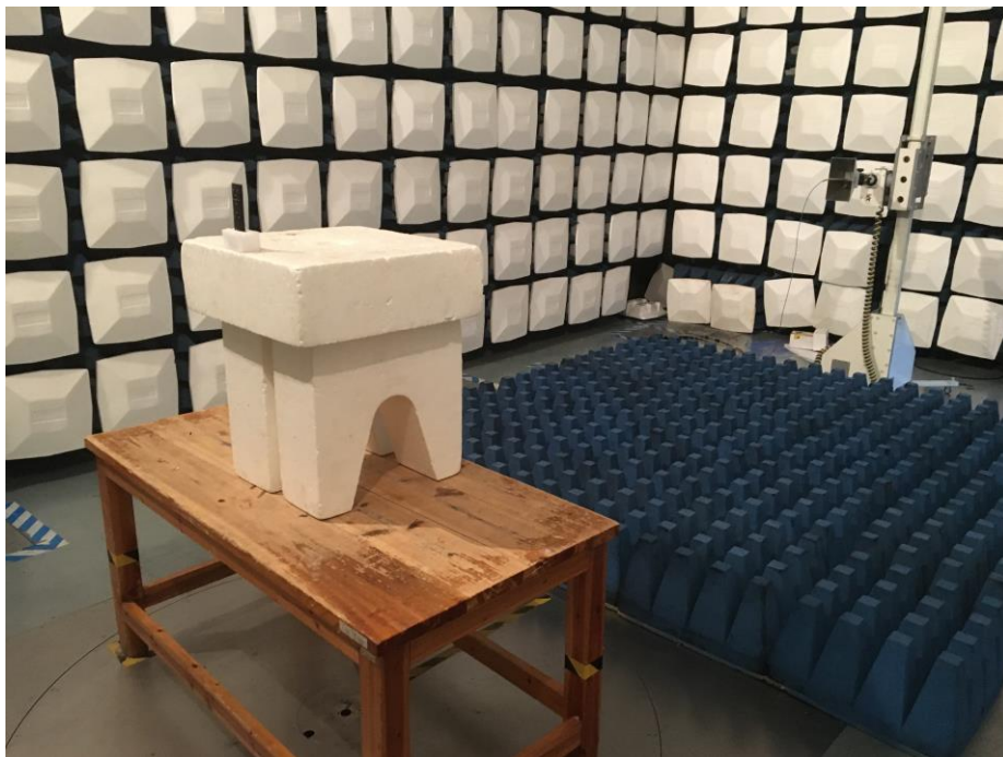
Test Setup For Radiated Emission (Above 1GHz)
