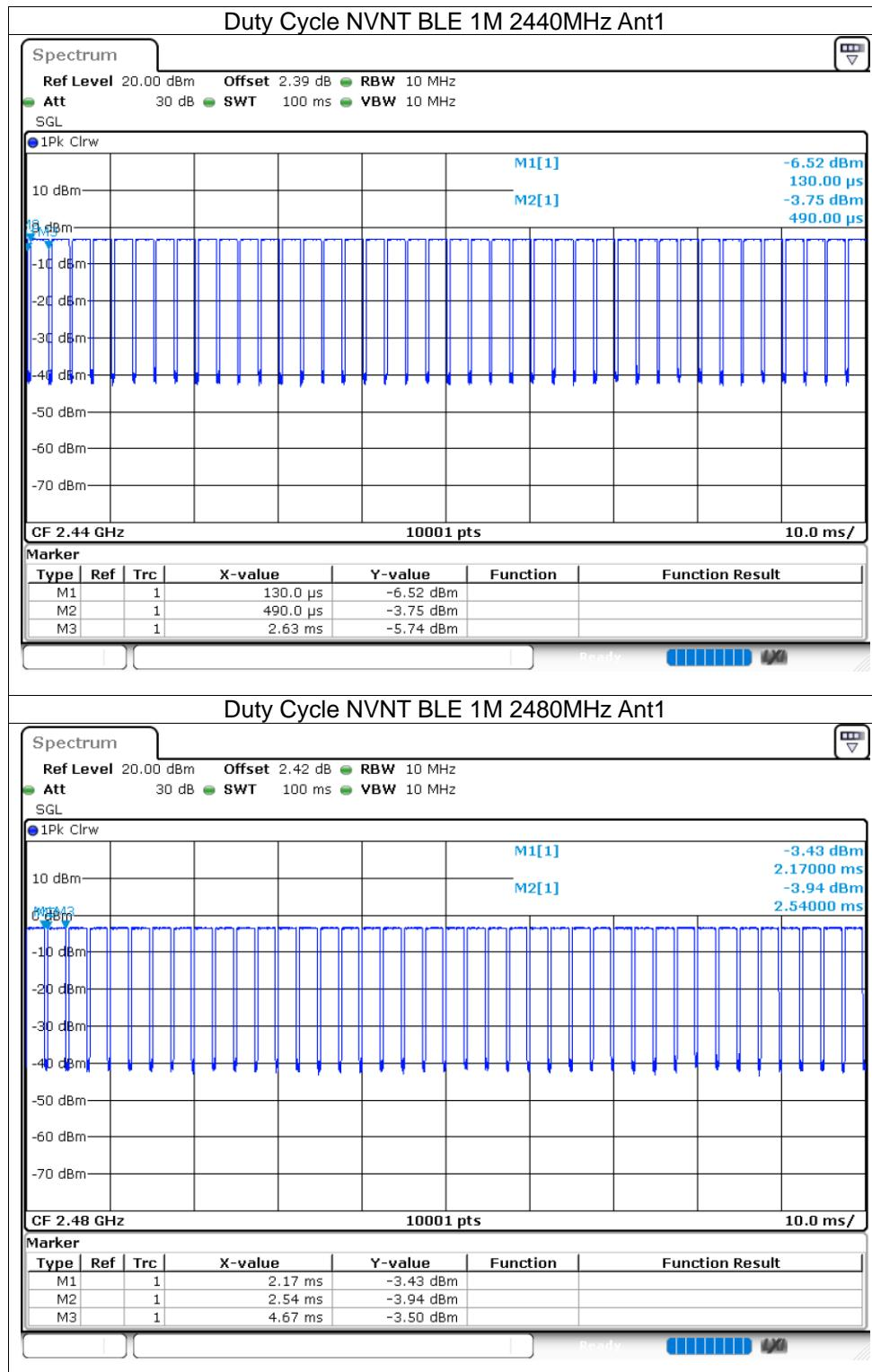
**Duty Cycle NVNT BLE 1M 2480MHz Ant1**
