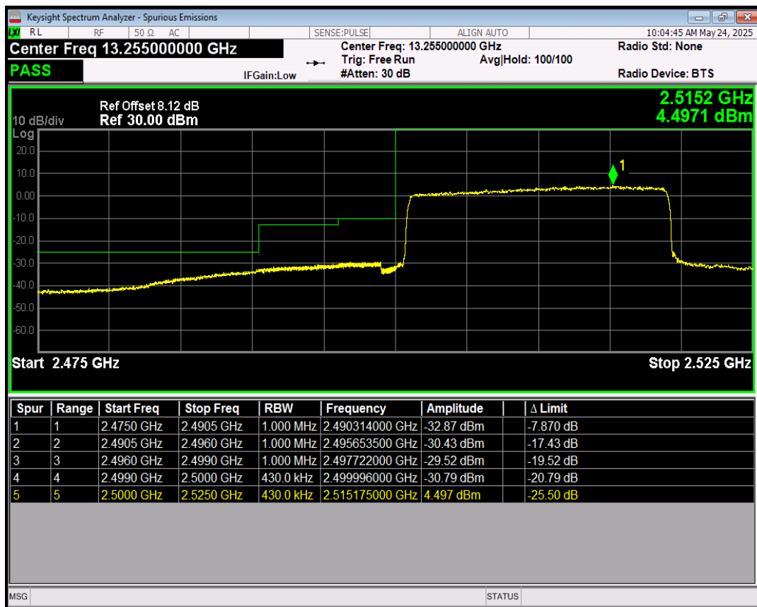
Band7 QPSK BW=20MHz Channel=21350 RB Size=1 Position=#0
