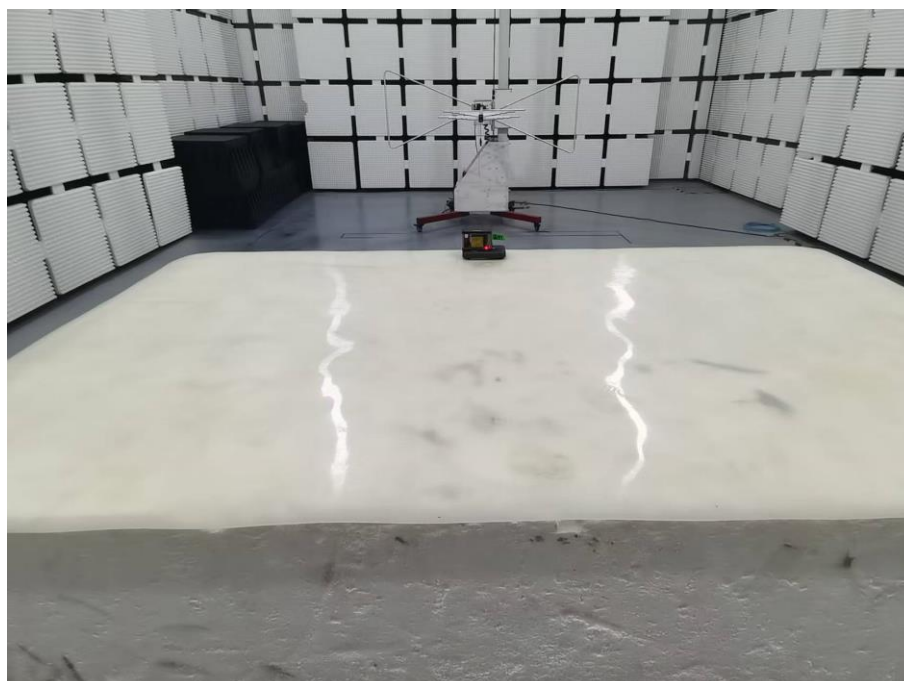
Photograph 2: Set-up photo for Radiated Emission, 30MHz - 1GHz
