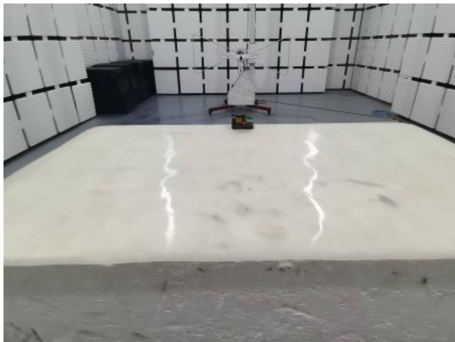
Photograph 2: Set-up photo for Radiated Emission, 30MHz - 1GHz
