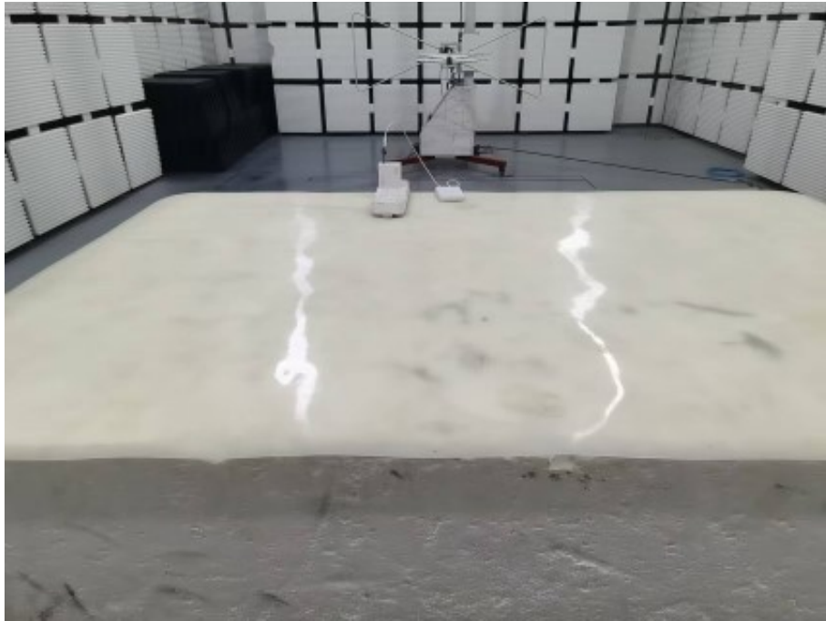
Photograph 2: Set-up photo for Radiated Emission, 30MHz - 1GHz
