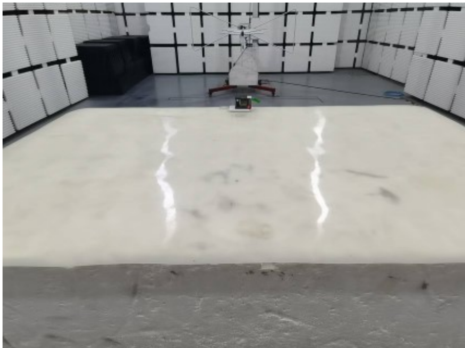
Photograph 2: Set-up photo for Radiated Emission, 30MHz - 1GHz
