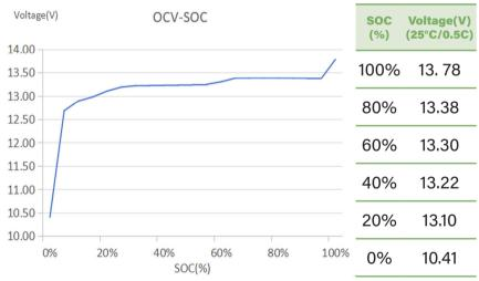
a: Based on the characteristics of LiFePO4 batteries, the voltage measured by all LiFePO4 batteries during charging/discharging is not the real voltage of the battery. Therefore, after charging/discharging and disconnecting the Battery from the power source, the voltage of the battery will gradually drop/increase to its real voltage.
