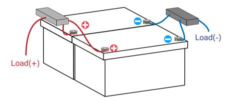
c: Connect Batteries Both in Series&Parallel Connect the batteries in parallel.
