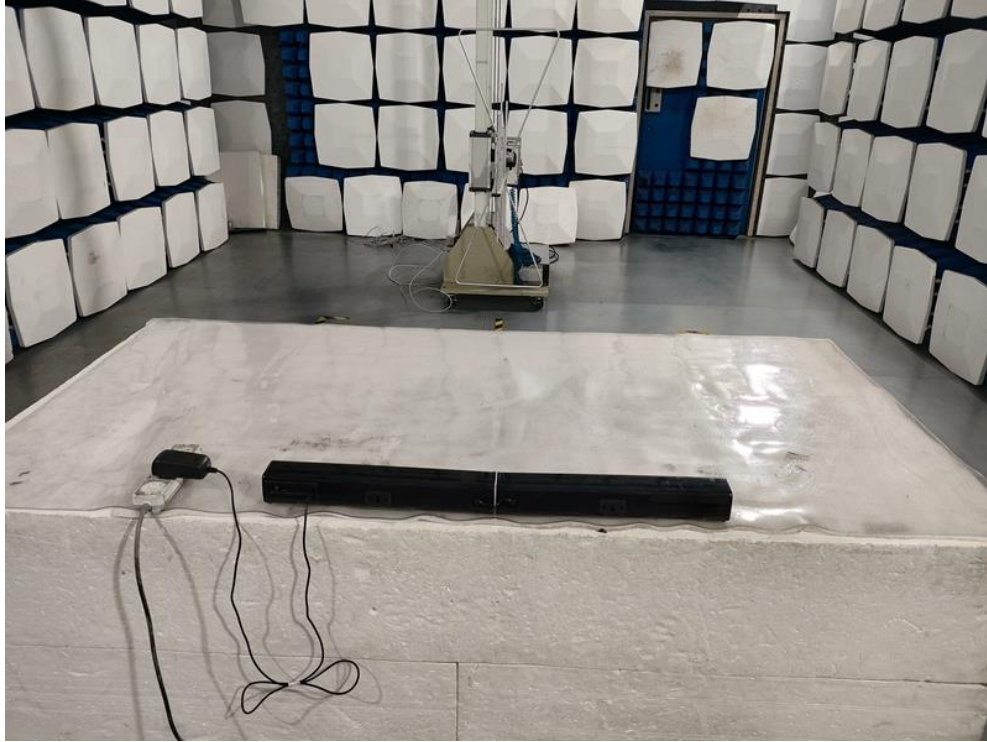
Radiated Emission Test Setup:
