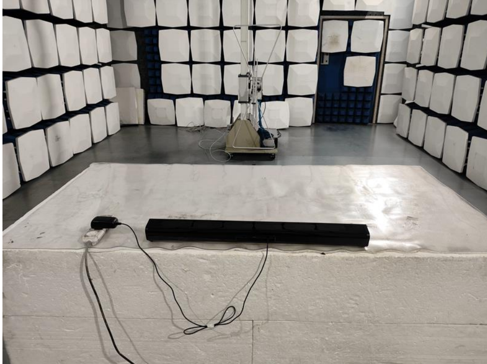
Radiated Emission Test Setup:
