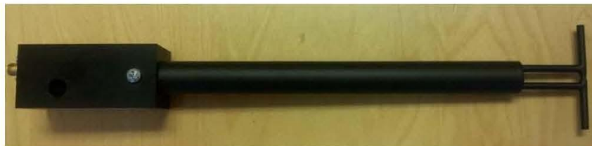
Figure 1 – MVG COMOSAR Validation Dipole
