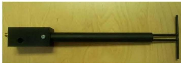
Figure 1 – MVG COMOSAR Validation Dipole
