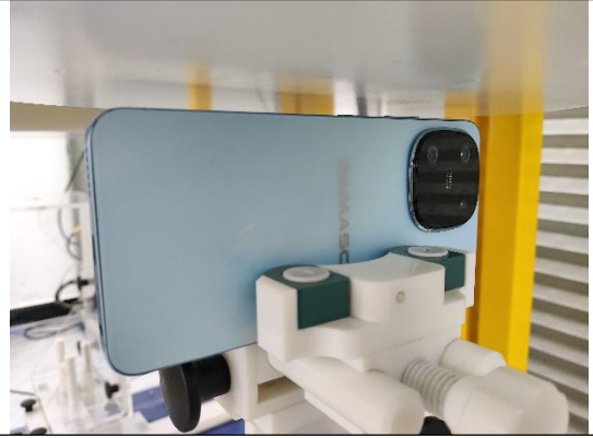
Bottom Side (Separation distance of 5mm)
