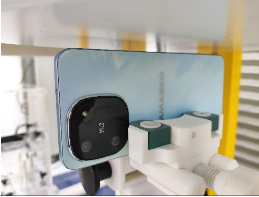
Top Side (Separation distance of 5mm)
