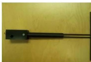
Figure 1 – MVG COMOSAR Validation Dipole
