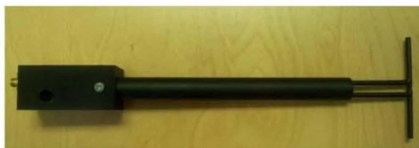
Figure 1 – MVG COMOSAR Validation Dipole
