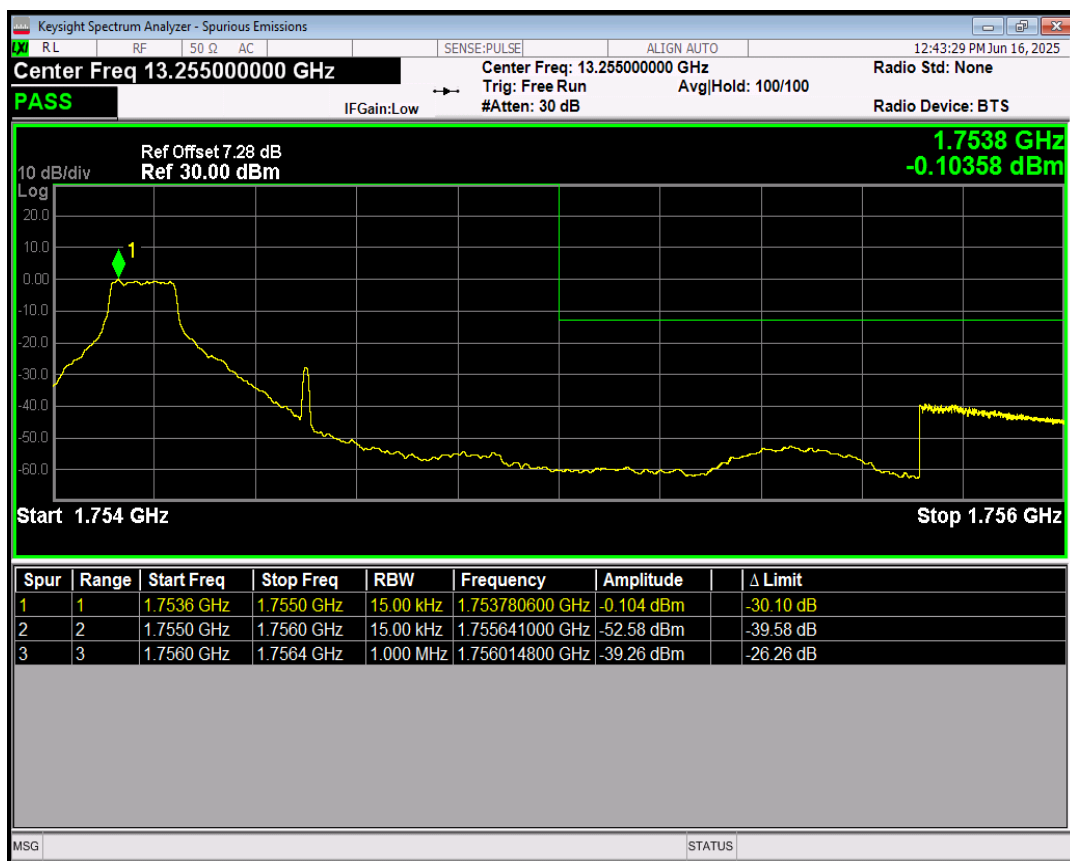
Band4 16QAM BW=1.4MHz Channel=20393 RB Size=1 Position=#Max
