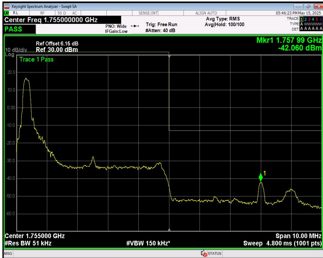
Band4 16QAM BW=5MHz Channel=20375 RB Size=1 Position=#0
