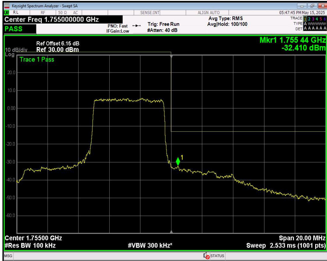
Band4 QPSK BW=10MHz Channel=20350 RB Size=25 Position=#Max
