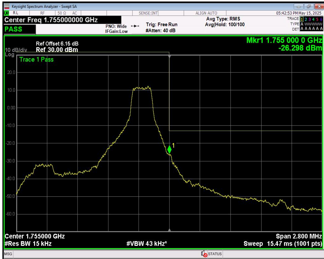
Band4 QPSK BW=1.4MHz Channel=20393 RB Size=1 Position=#Max
