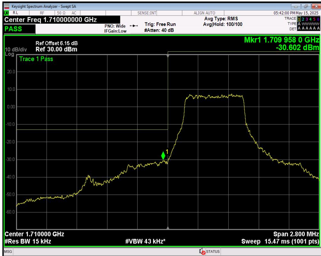
Band4 QPSK BW=1.4MHz Channel=19957 RB Size=3 Position=#0
