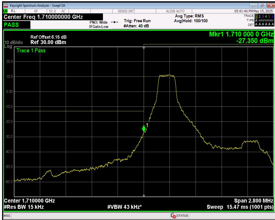
Band4 QPSK BW=1.4MHz Channel=19957 RB Size=1 Position=#0
