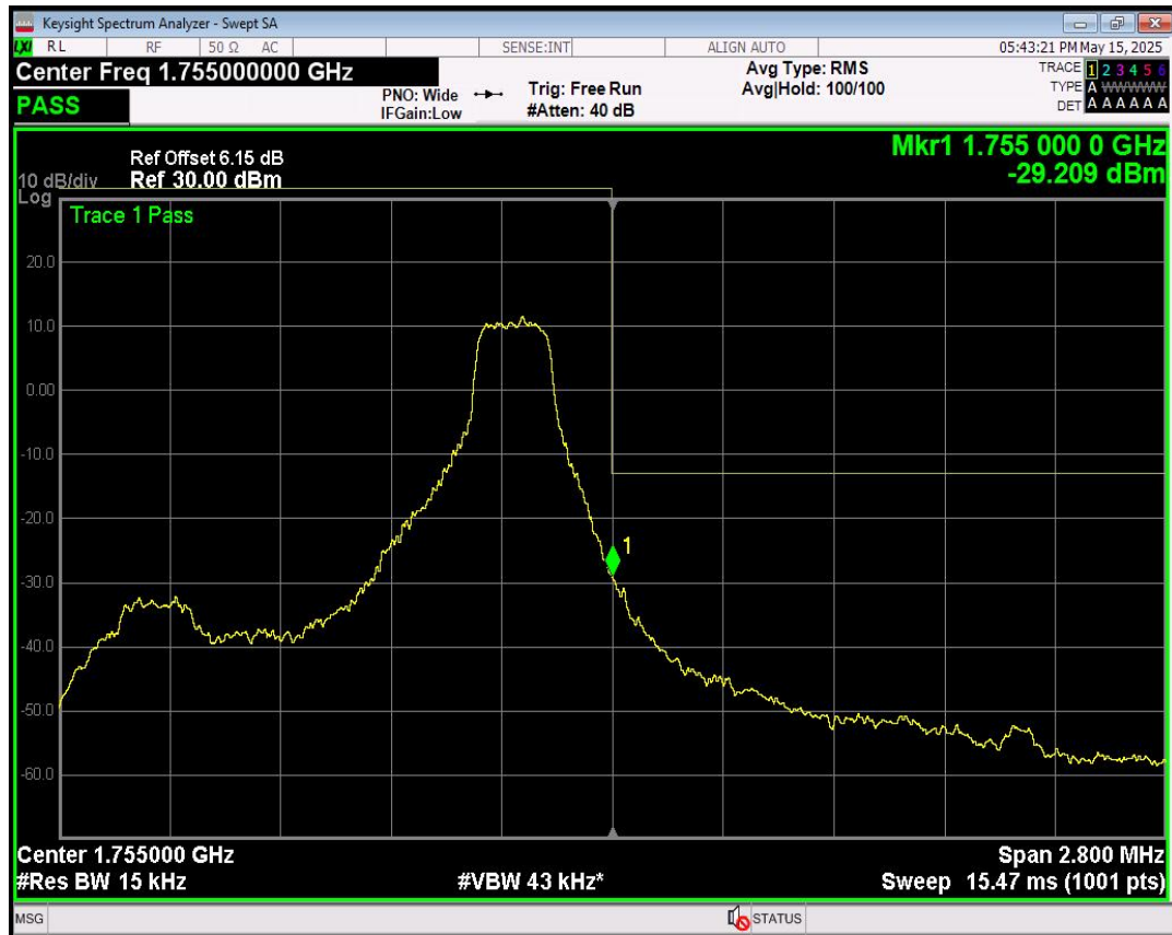
Band4 16QAM BW=1.4MHz Channel=20393 RB Size=1 Position=#Max
