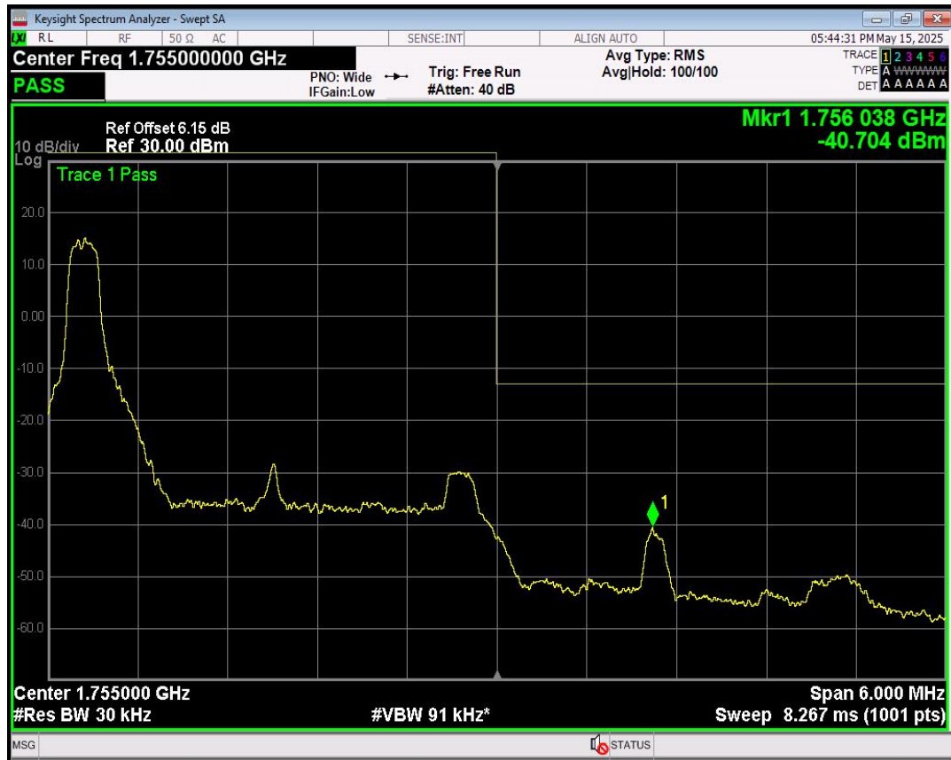
Band4 QPSK BW=3MHz Channel=20385 RB Size=1 Position=#0
