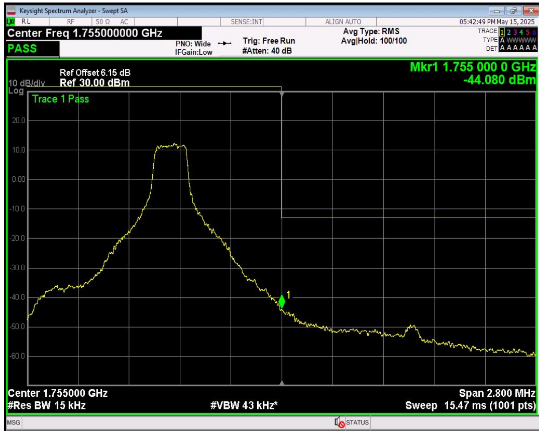
Band4 QPSK BW=1.4MHz Channel=20393 RB Size=1 Position=#Mid
