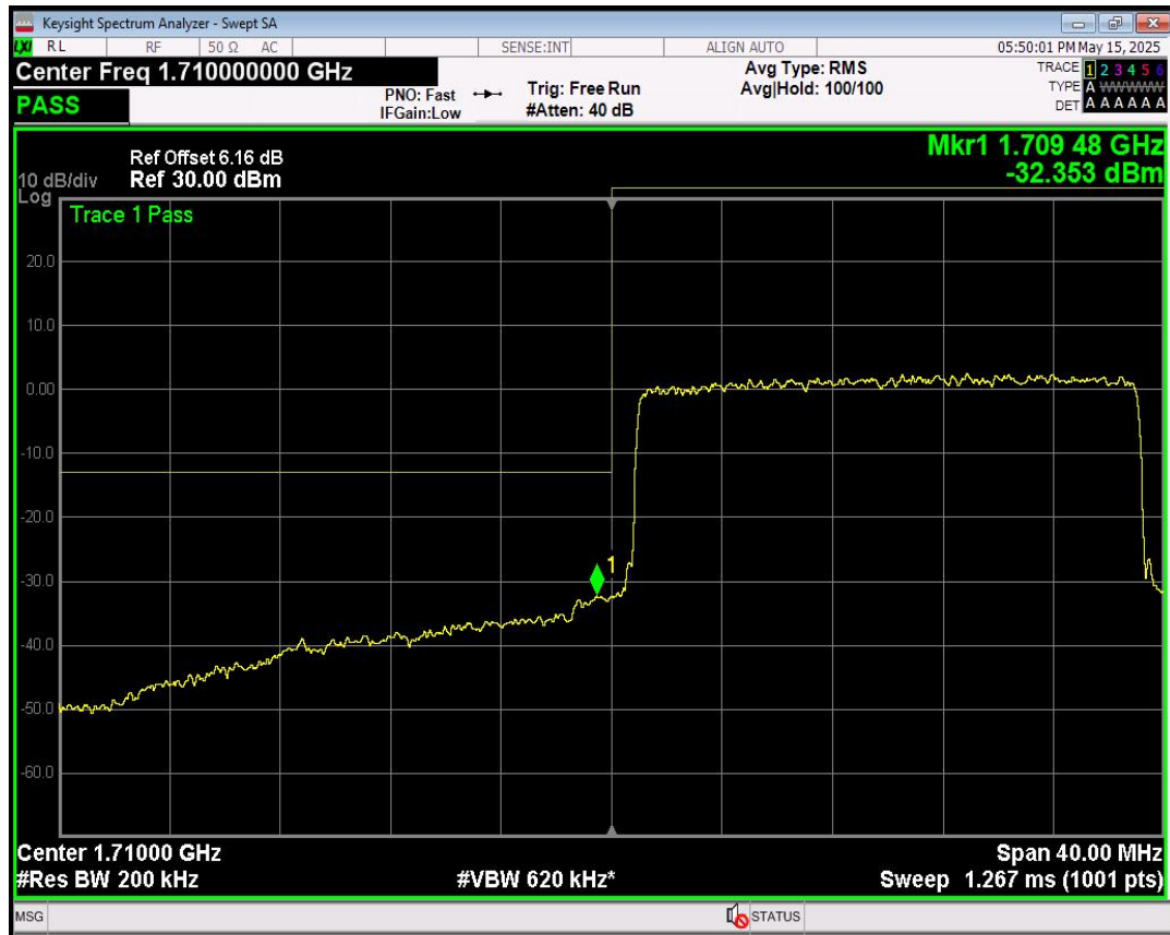
Band4 QPSK BW=20MHz Channel=20050 RB Size=100 Position=#0
