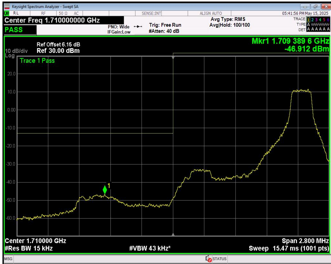
Band4 QPSK BW=1.4MHz Channel=19957 RB Size=1 Position=#Max
