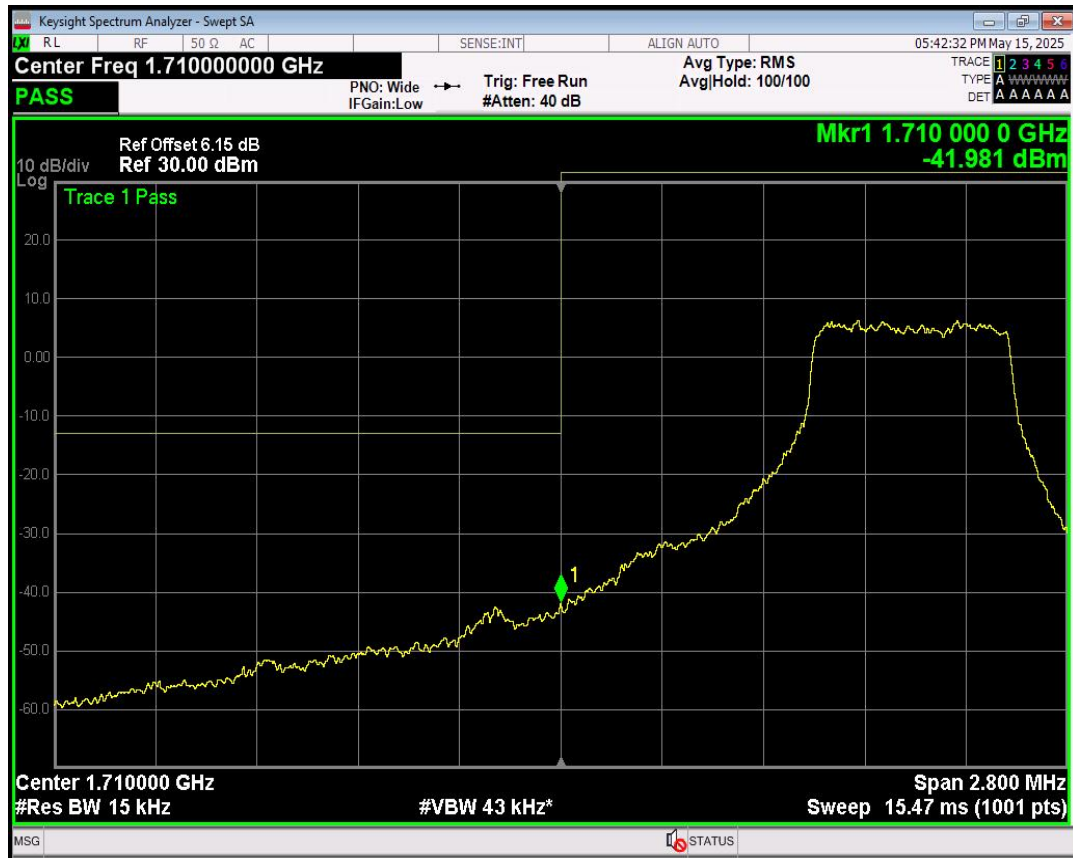
Band4 16QAM BW=1.4MHz Channel=19957 RB Size=3 Position=#Max
