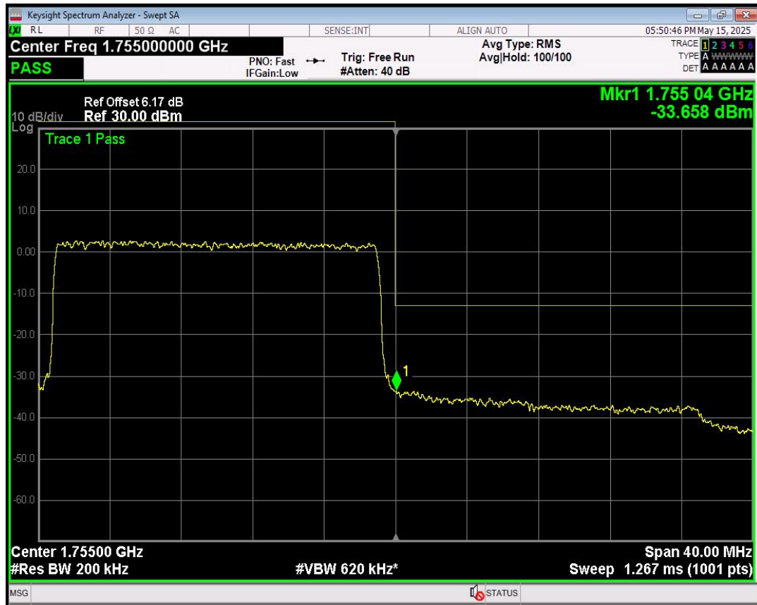
Band4 QPSK BW=20MHz Channel=20300 RB Size=100 Position=#0
