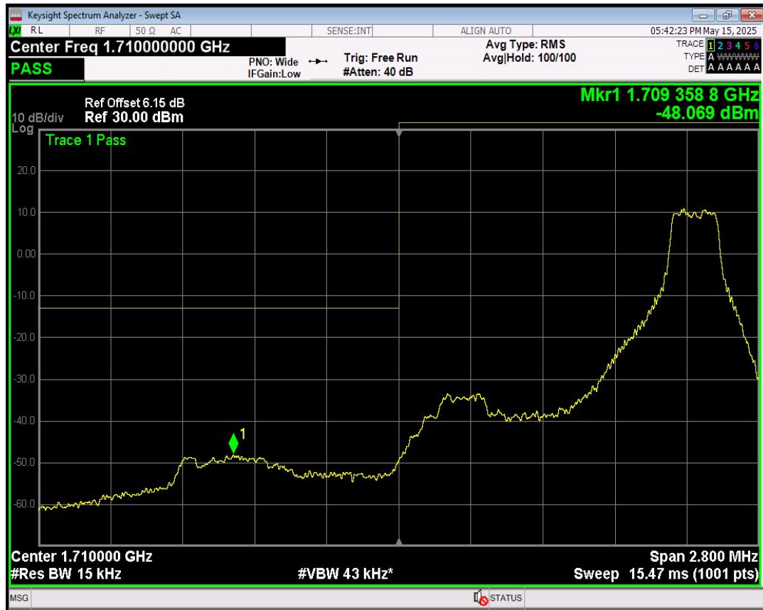
Band4 16QAM BW=1.4MHz Channel=19957 RB Size=1 Position=#Max
