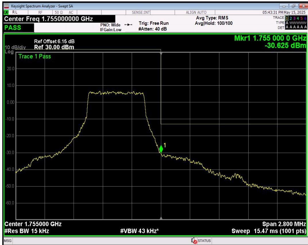
Band4 16QAM BW=1.4MHz Channel=20393 RB Size=3 Position=#Max
