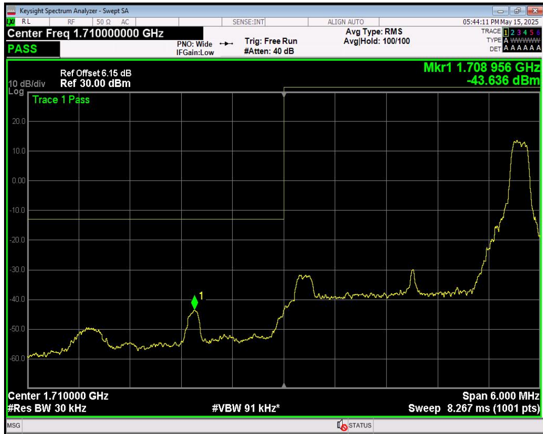
Band4 16QAM BW=3MHz Channel=19965 RB Size=1 Position=#Max
