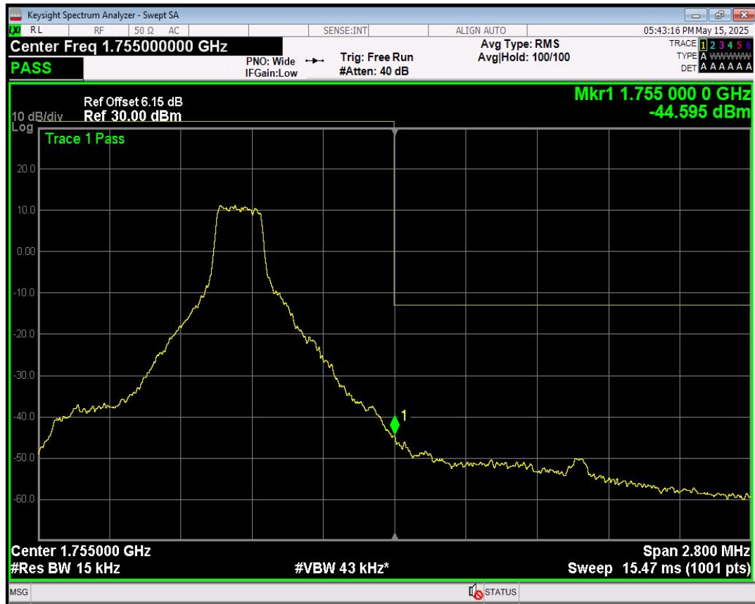
Band4 16QAM BW=1.4MHz Channel=20393 RB Size=1 Position=#Mid
