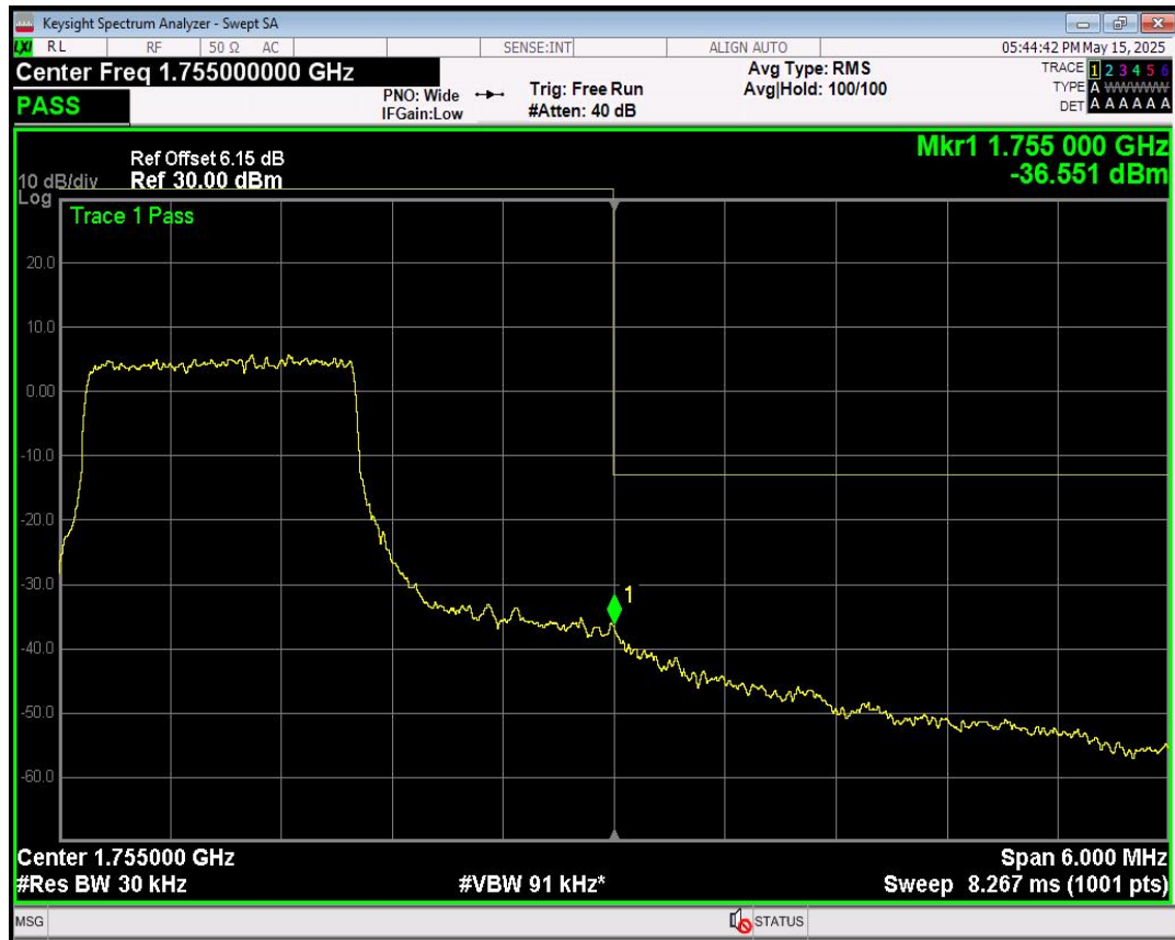
Band4 QPSK BW=3MHz Channel=20385 RB Size=8 Position=#0
