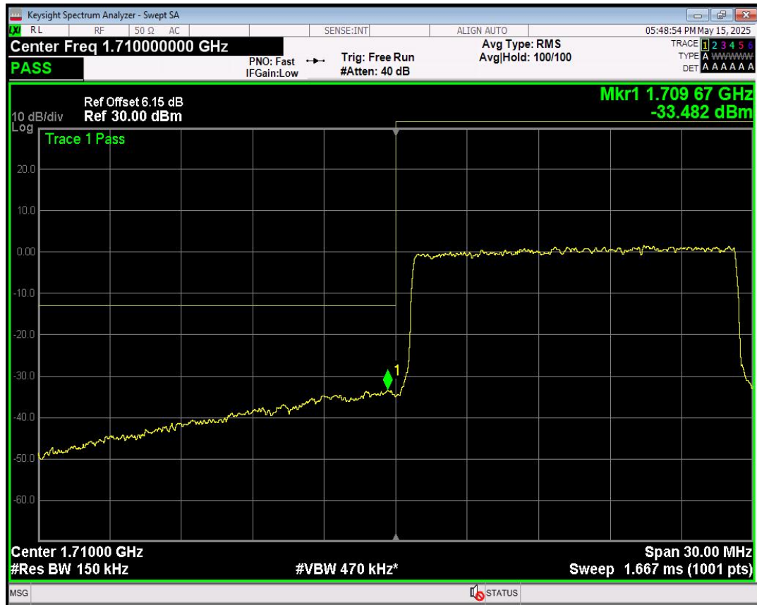
Band4 16QAM BW=15MHz Channel=20025 RB Size=75 Position=#0
