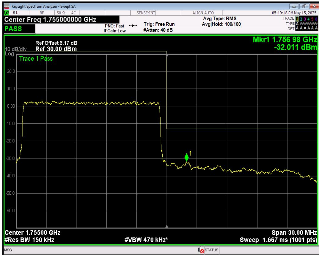
Band4 QPSK BW=15MHz Channel=20325 RB Size=75 Position=#0
