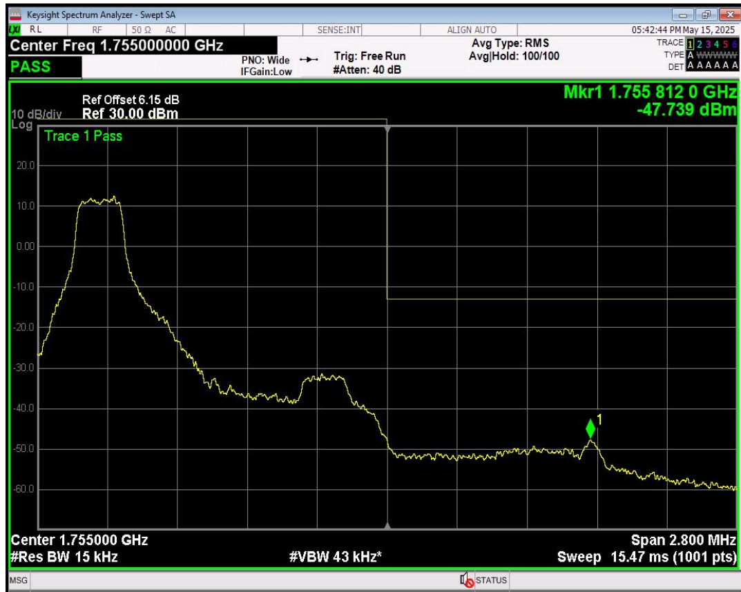
Band4 QPSK BW=1.4MHz Channel=20393 RB Size=1 Position=#0
