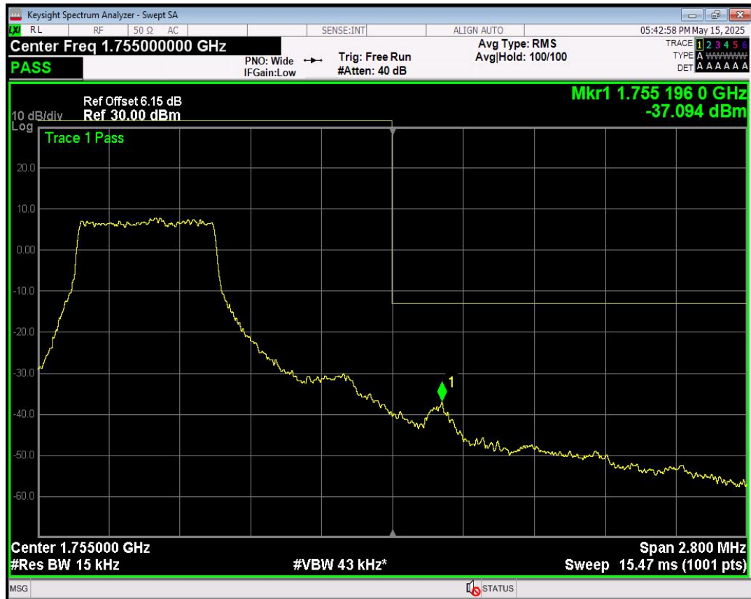
Band4 QPSK BW=1.4MHz Channel=20393 RB Size=3 Position=#0
