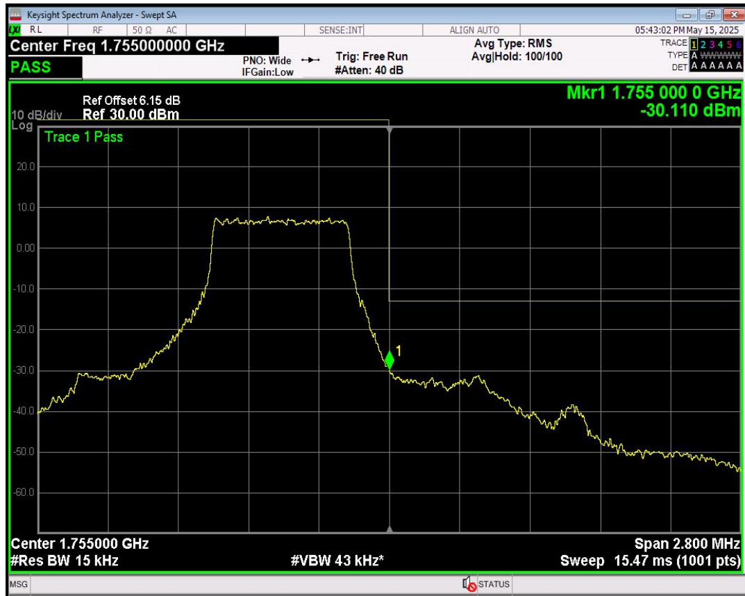
Band4 QPSK BW=1.4MHz Channel=20393 RB Size=3 Position=#Max
