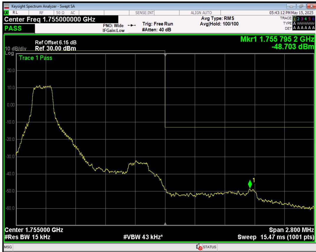
Band4 16QAM BW=1.4MHz Channel=20393 RB Size=1 Position=#0
