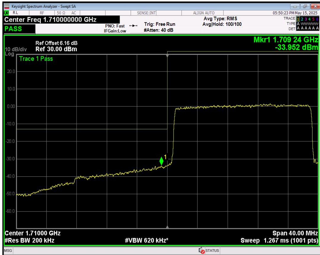
Band4 16QAM BW=20MHz Channel=20050 RB Size=100 Position=#0
