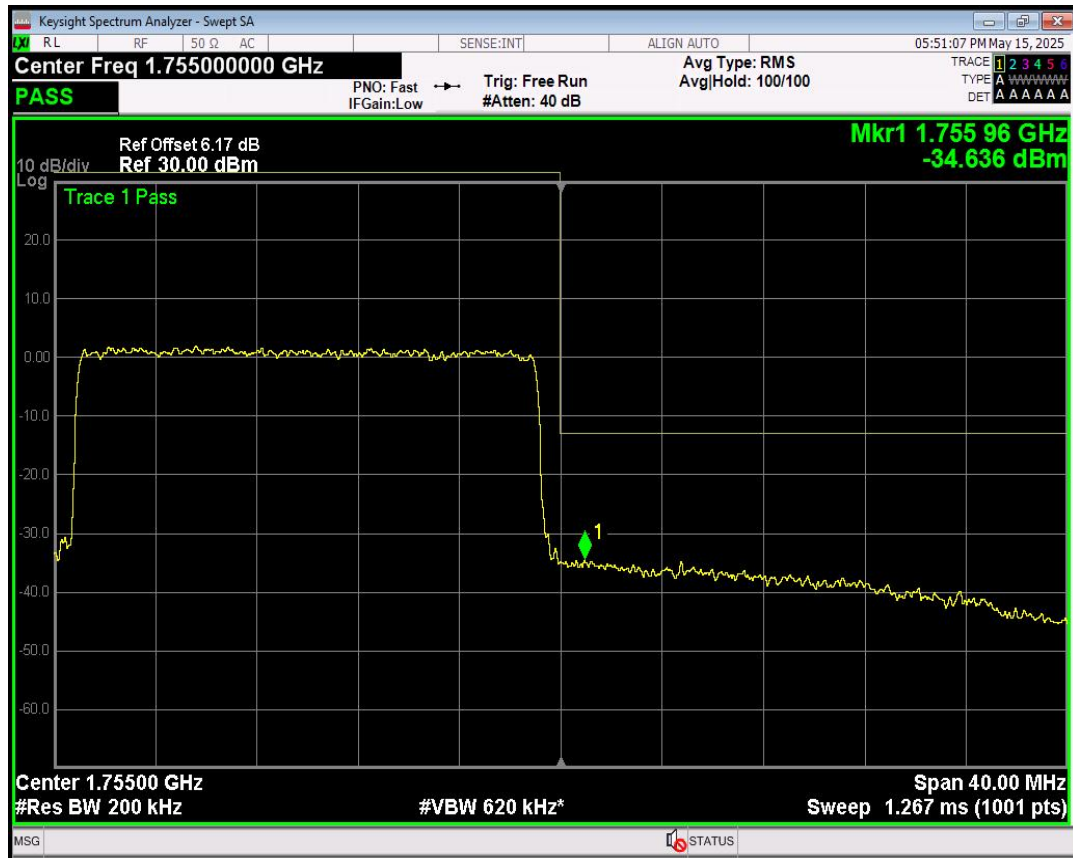
Band4 16QAM BW=20MHz Channel=20300 RB Size=100 Position=#0
