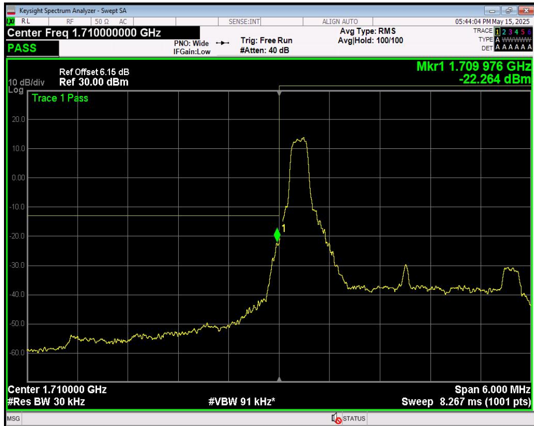
Band4 16QAM BW=3MHz Channel=19965 RB Size=1 Position=#0
