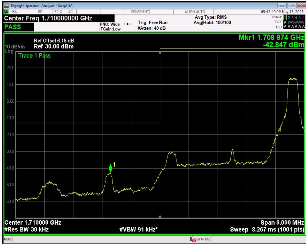
Band4 QPSK BW=3MHz Channel=19965 RB Size=1 Position=#Max
