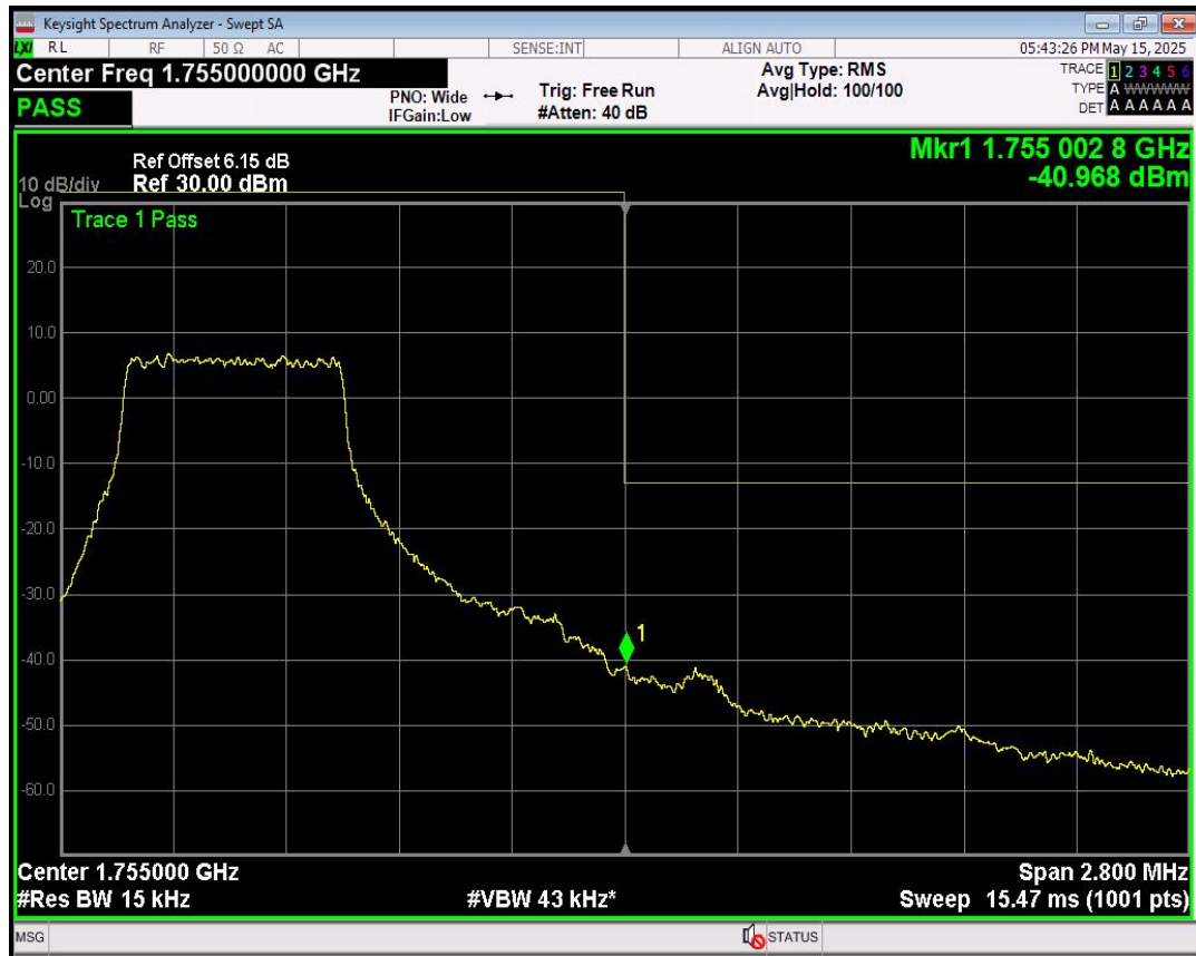
Band4 16QAM BW=1.4MHz Channel=20393 RB Size=3 Position=#0
