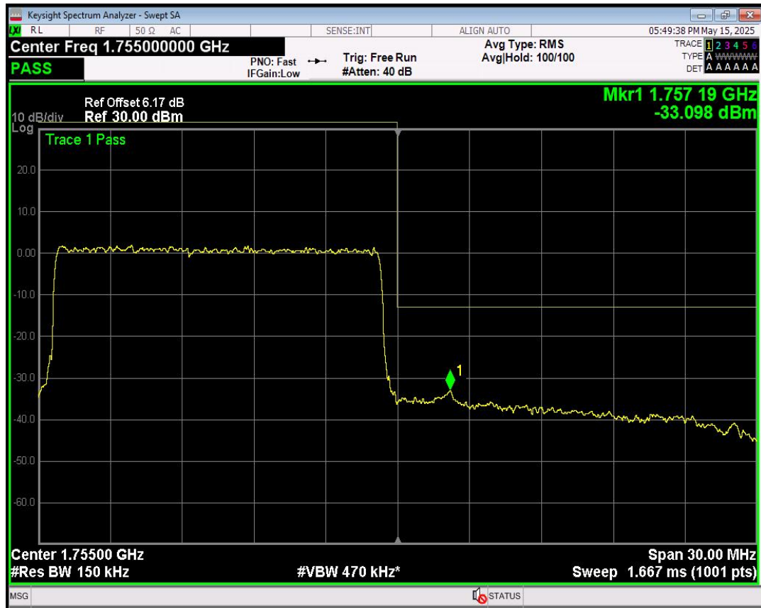
Band4 16QAM BW=15MHz Channel=20325 RB Size=75 Position=#0
