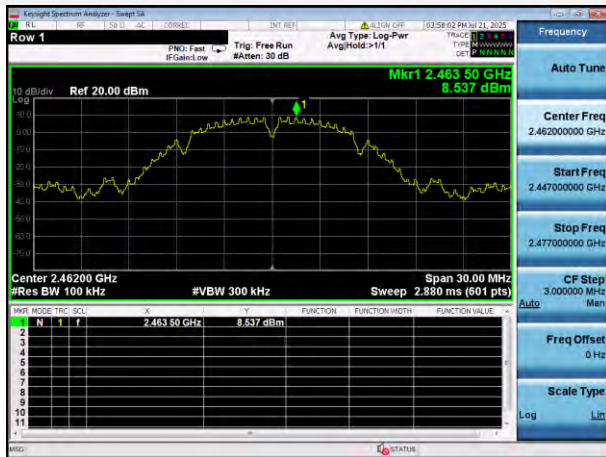
802.11b HIGH CHANNEL, CARRIER LEVEL
