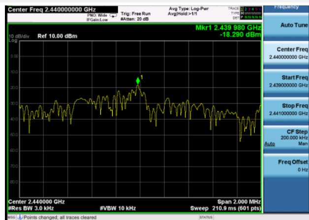
GFSK (BLE 2Mbps) MIDDLE CHANNEL
