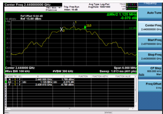
GFSK (BLE 2Mbps) MIDDLE CHANNEL
