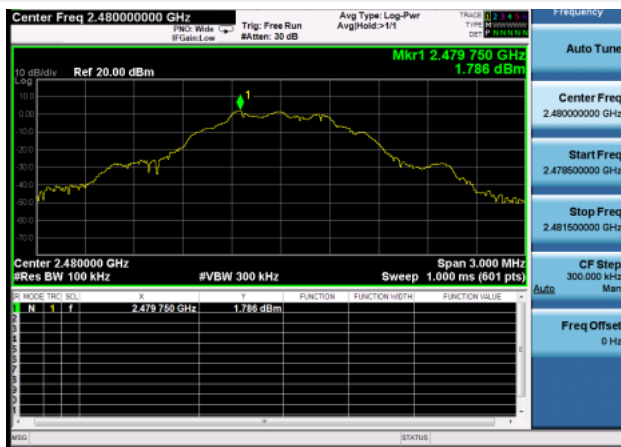
GFSK (BLE 1Mbps) HIGH CHANNEL, CARRIER LEVEL
