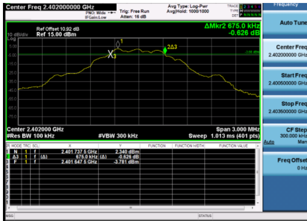
GFSK (BLE 1Mbps) LOW CHANNEL
