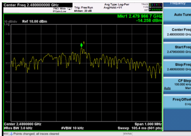
GFSK (BLE 1Mbps) HIGH CHANNEL
