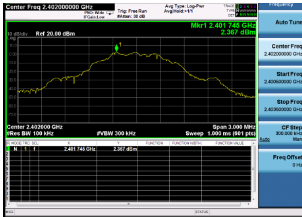
GFSK (BLE 1Mbps) LOW CHANNEL, CARRIER LEVEL
