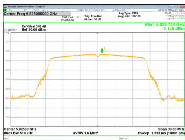
(802.11a) PSD plot on channel 165
