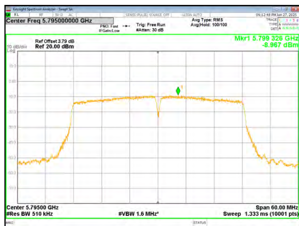
(802.11ac40) PSD plot on channel 151
