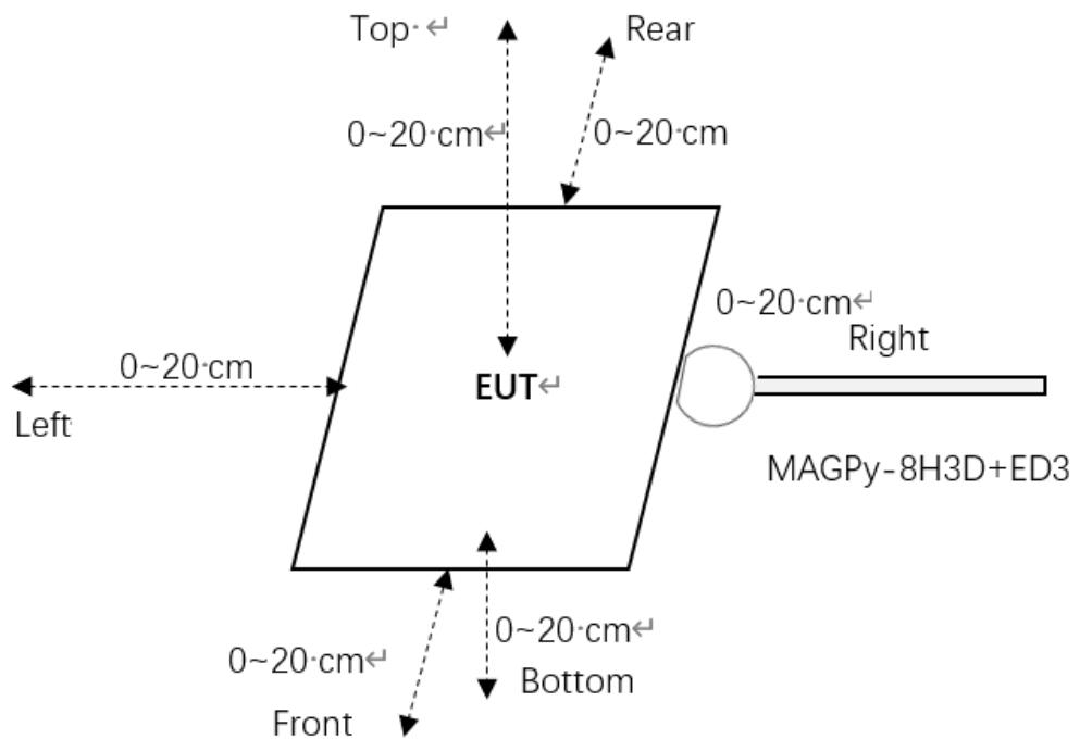
Note: tips mode of the test probe is used for 0cm measurement.
