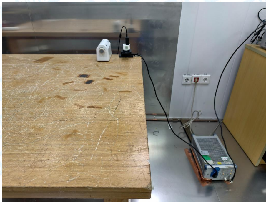
Radiated Emission Test Setup-Below 1G
