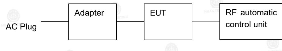
The sample was placed (0.8m below 1GHz, 1.5m above 1GHz) above the ground plane of 3m chamber. Measurements in both horizontal and vertical polarities were performed.
