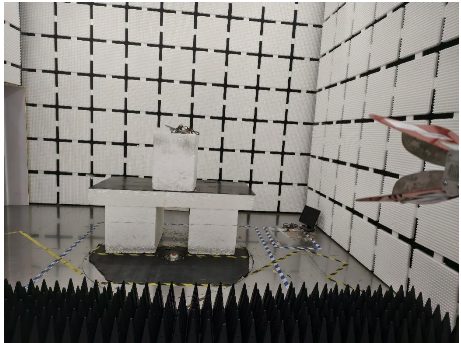
Radiation Emission Test Setup (1GHz to 18GHz)
