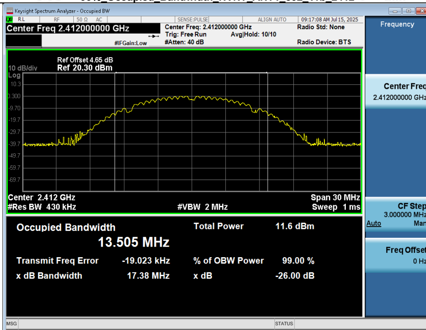
99% Occupied Bandwidth NVNT ANT1 802_11b 2412
