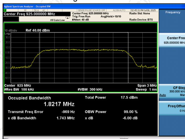
802.11ah 16QAM Modulation
