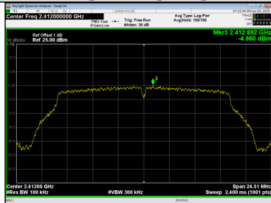
In-Band Reference Level IEEE 802.11g_Channel 1_20MHz_Antenna 0
