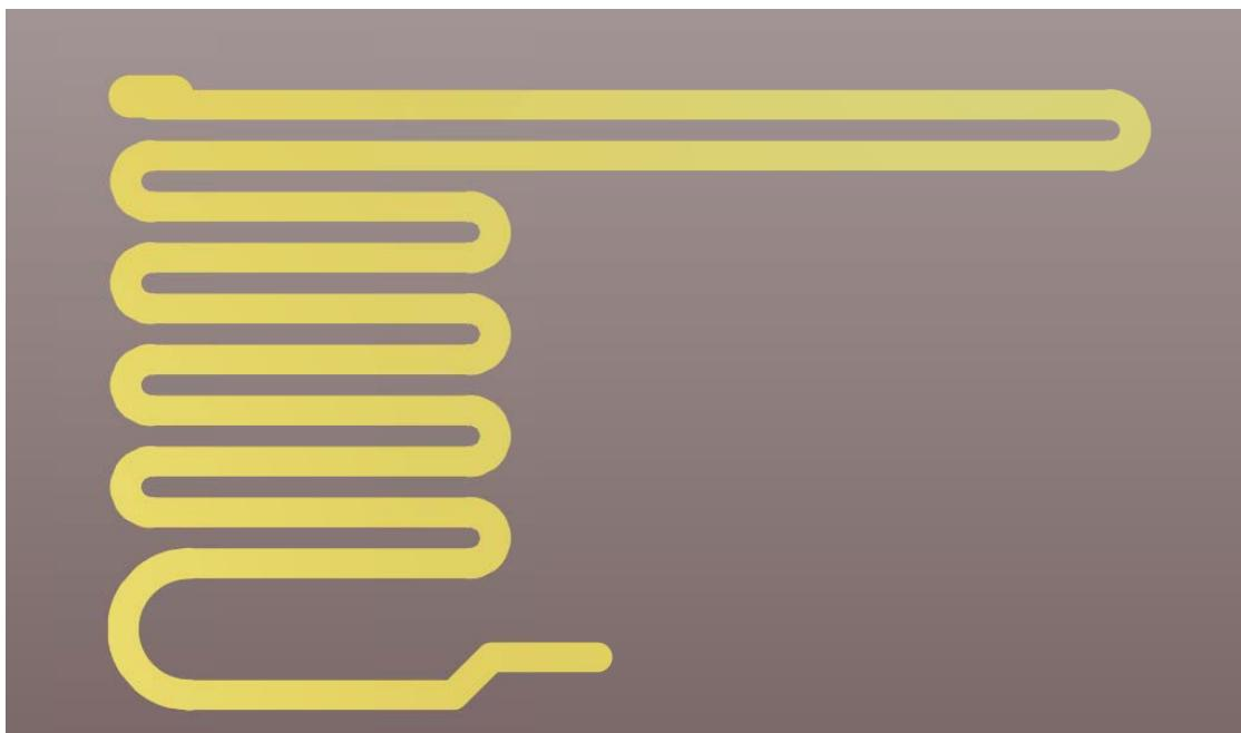
Antenna model : PCB On-board antennas
