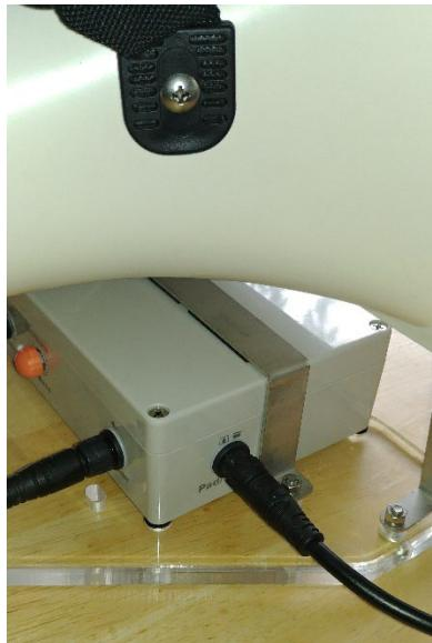
The cable should connect firmly into the speaker socket
