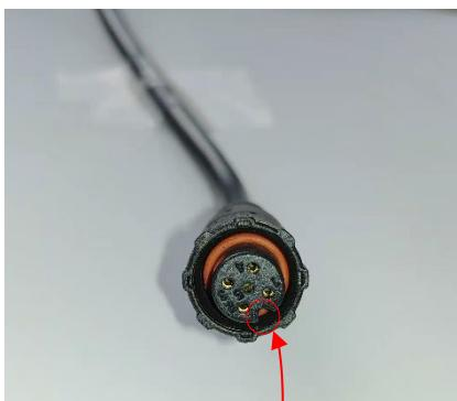
Take note that the small grooves line up before inserting cable into socket
