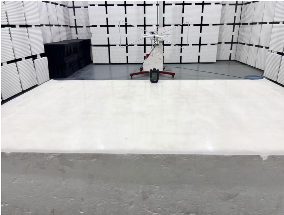
Set-up for Radiated Spurious Emission, Above 1GHz
