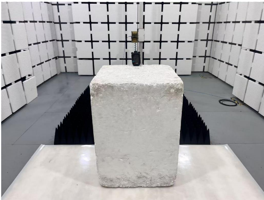
Set-up for Radiated Spurious Emission, Above 1GHz
