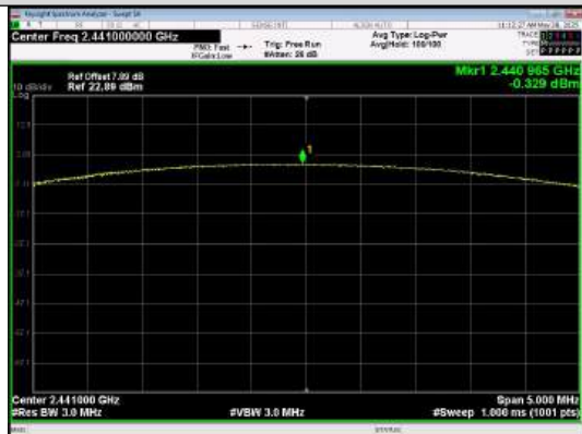
Peak Output Power n/4DQPSK_Channel 39
