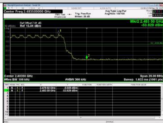
Out Of Band Emission(Right) π/4QPSK_2-DH1_Channel Hopping
