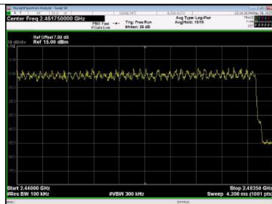
High End Spectrum Channel Hopping Plot 8DPSK
