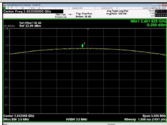
Peak Output Power 8DPSK_Channel 0
