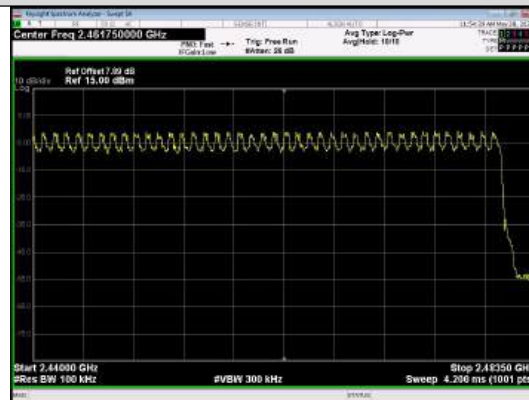
High End Spectrum Channel Hopping Plot n/4DQPSK
