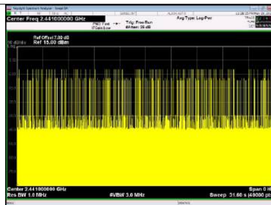
Number of Pulses in 31.6 seconds GFSK_DH5
