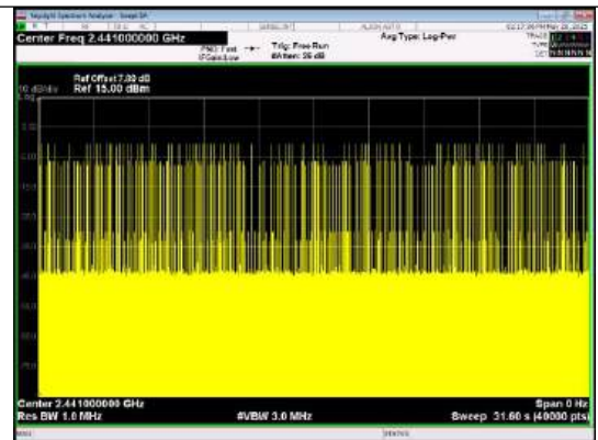
Number of Pulses in 31.6 seconds 8DPSK_3-DH5
