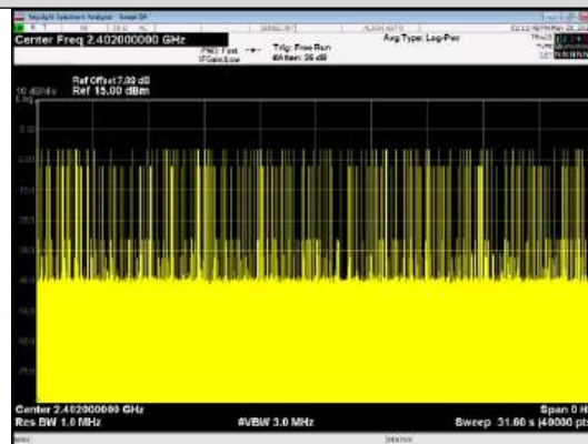
Number of Pulses in 31.6 seconds n/4DQPSK_2-DH5
