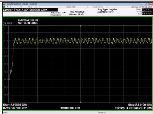
Low End Spectrum Channel Hopping Plot n/4DQPSK
