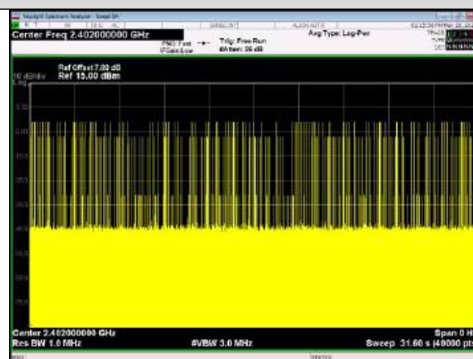
Number of Pulses in 31.6 seconds 8DPSK_3-DH5
