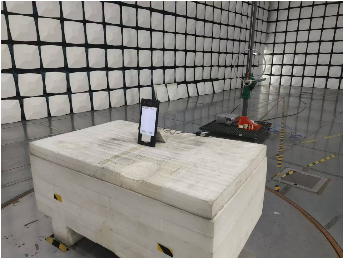
Radiated Emission 9k-30MHz Perpendicular View
