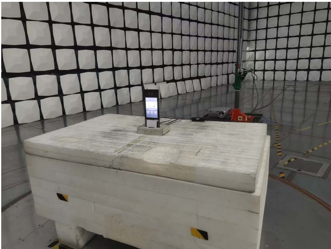
Radiated Emission 9k-30MHz Perpendicular View
