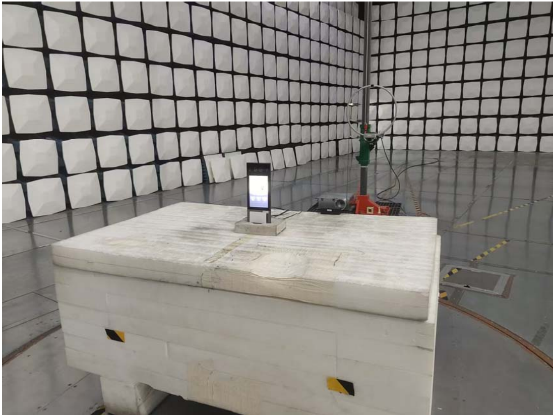
Radiated Emission 9k-30MHz Perpendicular View
