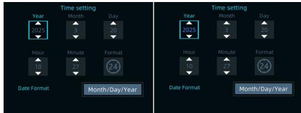
Operation method: Press the to go to the time setting interface, press the button or the button to select year, month, date, hour, and minute, then press the button to confirm the selection, and the icon will light up. Then press the button or the button to set values. After selection, press the button to cancel the selection, and the icon will become dimmer.
